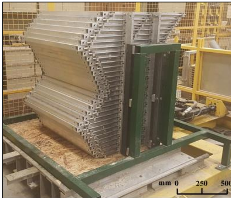
Figure 3.3 Flexible Laminar Shear Box (FLSB) developed and built for this study
