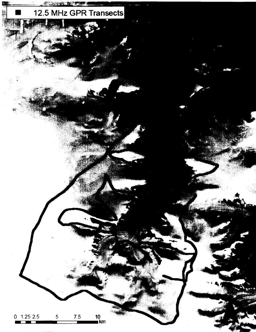
Figure 3.6: Locations of 12.5Mhz GPR surveys taken during the May 2008 field season (combined with other datasets) to develop the BedDEM of Belcher Glacier.
