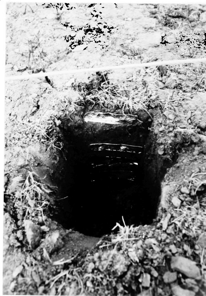
Figure 3.7 Solifluction measurements: A) Painted pebbles, Slope 5, July 1984; B) Tin foil markers being inserted, Slope N, July 1984.
