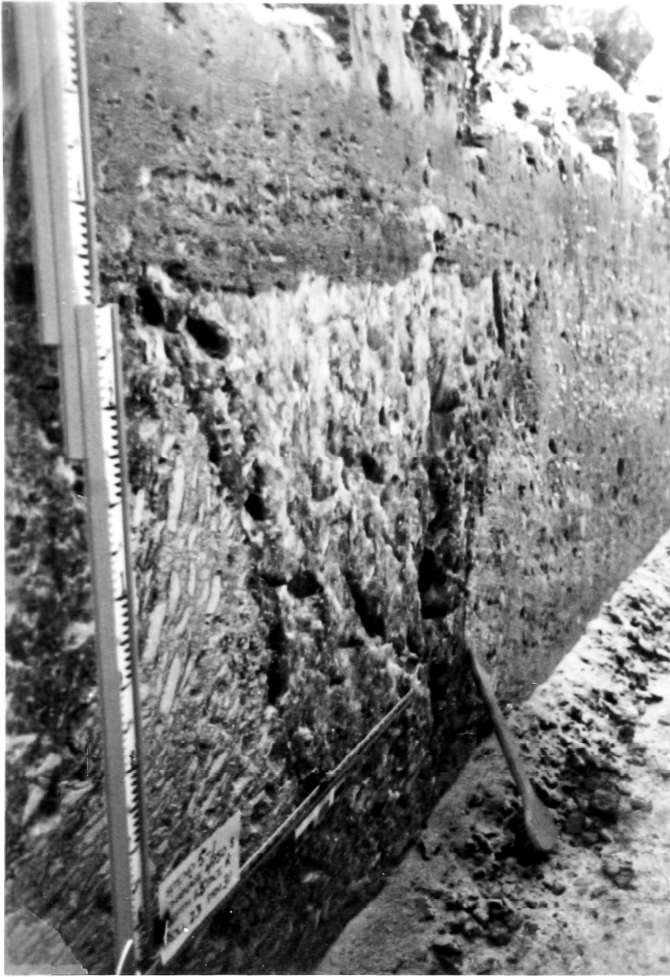
Figure 4.2 Observations in EBA trenches excavated in Weatherall Formation sandstone, winter 1981-82: A) Large ice wedge in Trench 5. Note bending of colluvium at side of wedge. B) Bending of vertically-oriented Weatherall siltstone strata at colluvium/residuum contact in trench 5. (Photos courtesy of EBA Engineering.)
