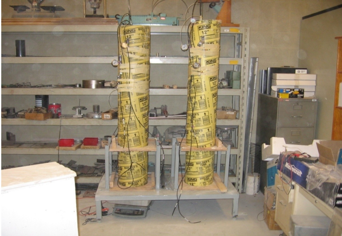
Figure 5-2 Set-up of columns (drained (D; to the left), and undrained (UN; to the right), conditions)
