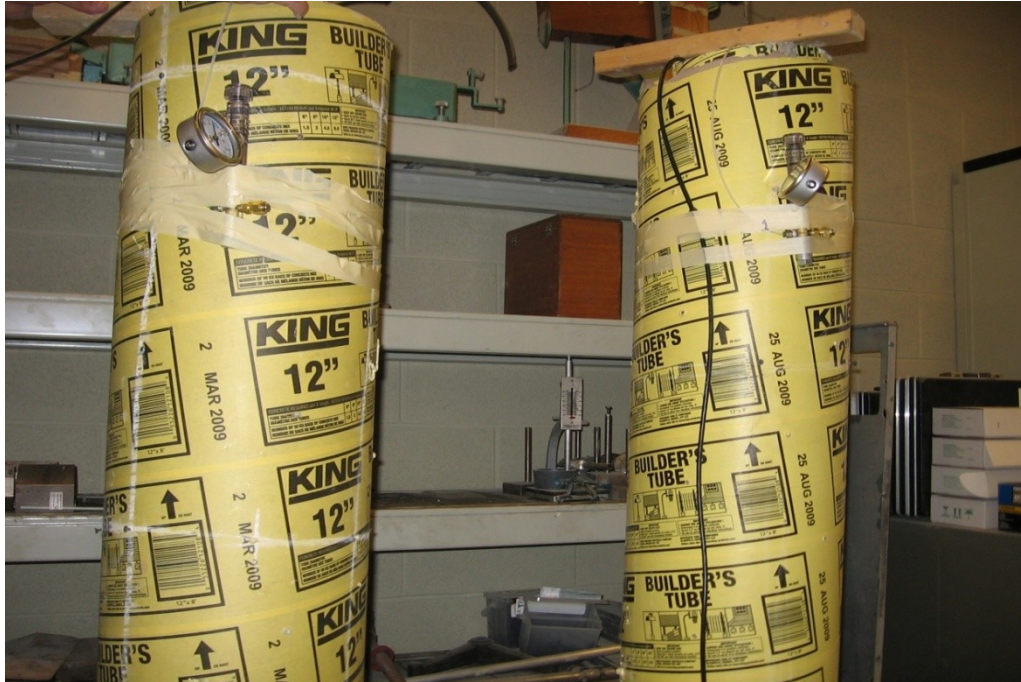
Tensiometers fixed on the columns
