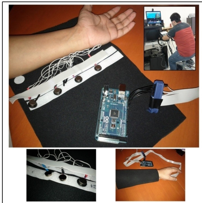
Figure 5.19 The arm bands with actuators in position and user (top right) blindfolded playing the game
