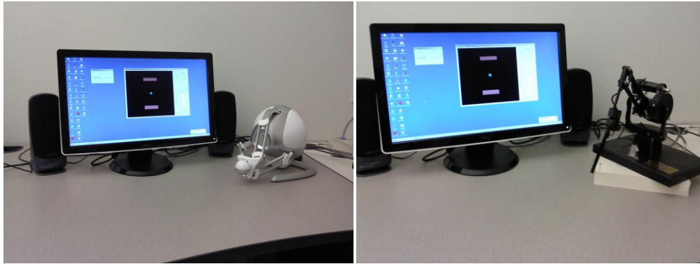
Figure 3.1 Technical setup with Falcon (left) and Phantom (right) devices
