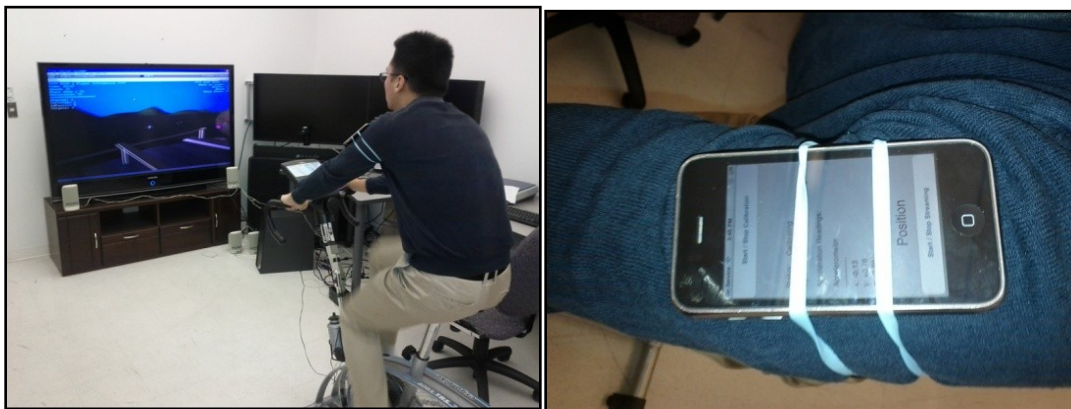
Figure 5.7 “Move-tilt” application running on the smartphone, attached to the player’s arm
