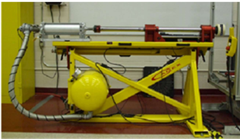
Study 1 - Figure 1: Linear Impactor
