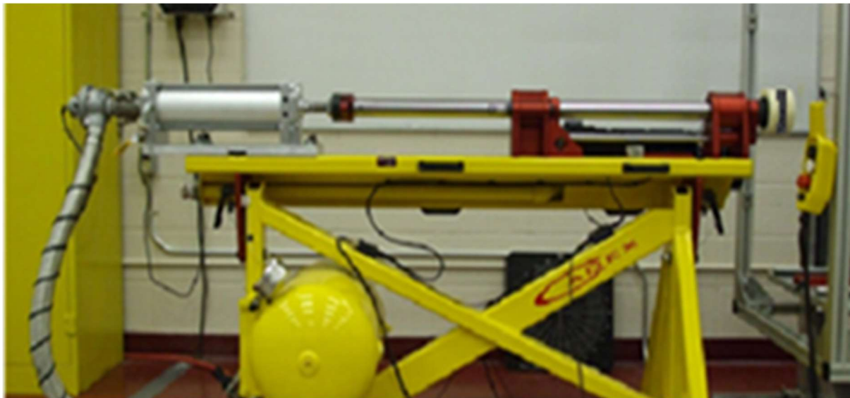
Study 3 - Figure 2: Linear Impactor
