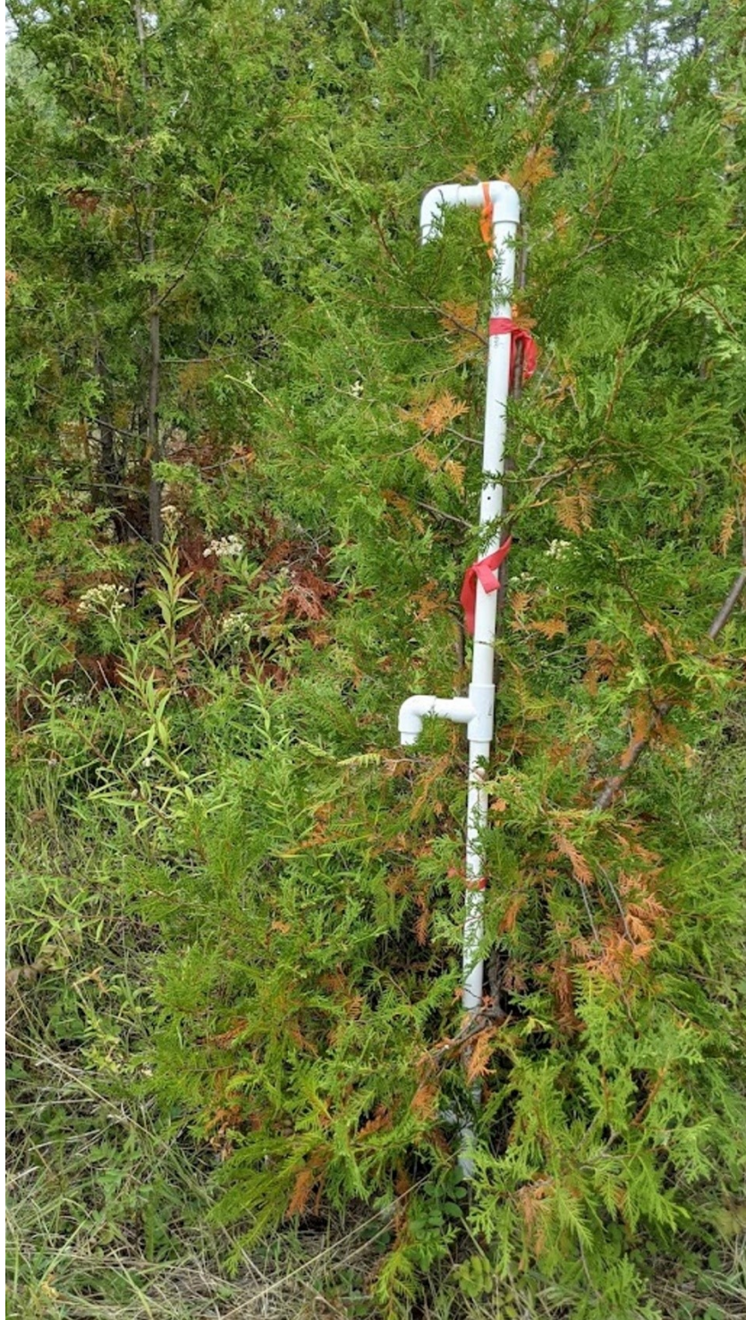
Figure 1.1. Image of a PVC pole containing iButtons at 0.05 m, 0.75 m, and 1.5 m deployed in the field. Photo credit: Gabrielle Ednie.
