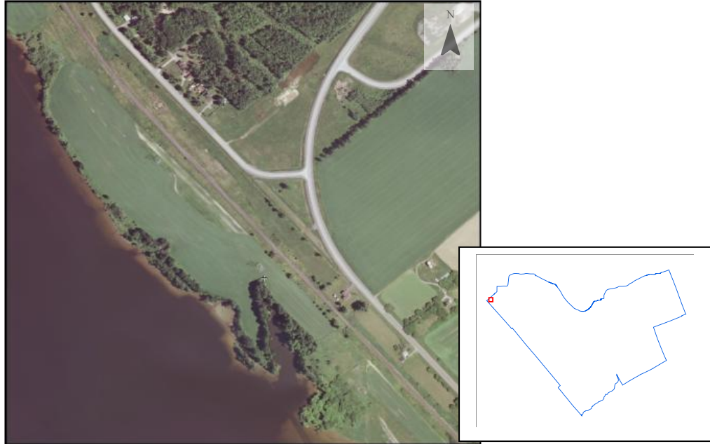
Figure 2.3: One tile of ortho-rectified, multispectral aerial imagery over western Ottawa at a resolution of 20x20cm. Source: Ontario Ministry of Natural Resources (see text for full explanation).
