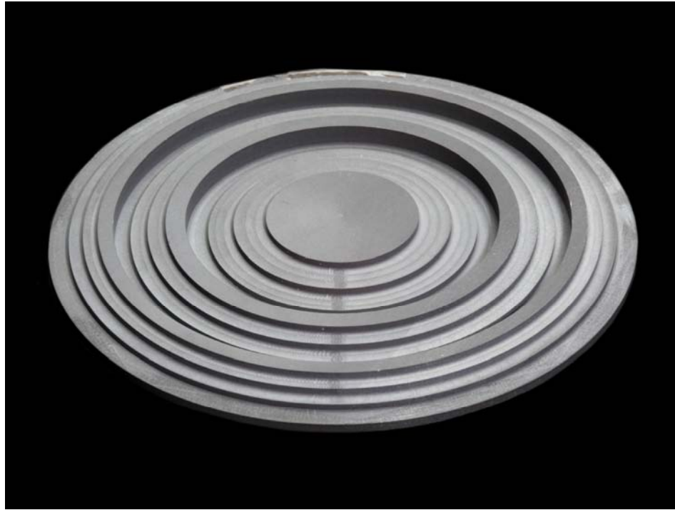
Figure 6.3-2: Dielectric phase-correcting Fresnel zone plate antenna (PC-FZPA).
