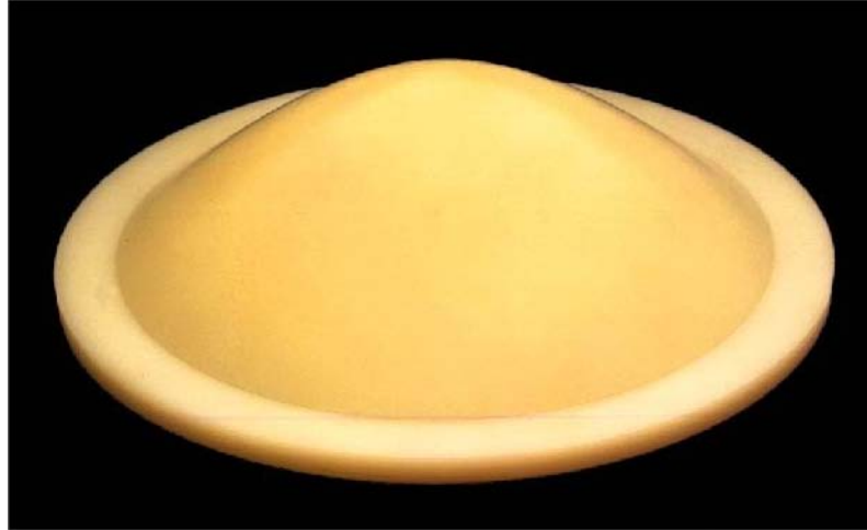
Figure 2.3-1: Dielectric plano-hyperbolic lens antenna (courtesy of CRC).
