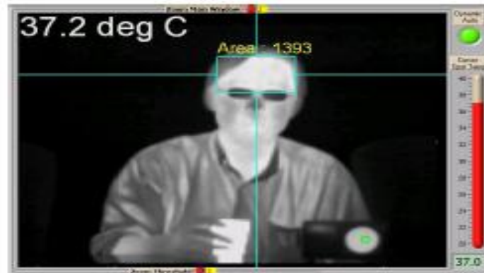
Figure 2.5: Thermal image of a person taken by type four thermal imaging system with core body temperature indication [13].
