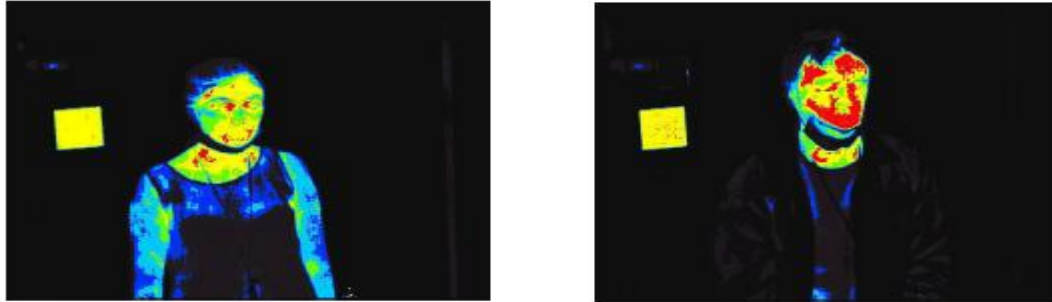
Figure 2.3: Thermal images taken by type one thermal imaging systems using a square shaped temperature reference source, image on the left shows a person with normal temperature and image on the right is a person with fever [13].
