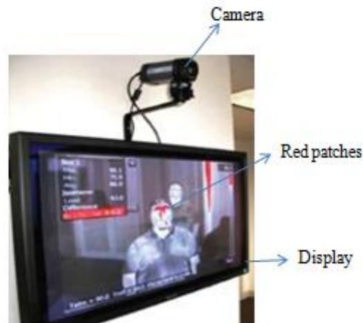
Figure 2.9: FLIR thermal imaging setup used in mass fever screening [18].
