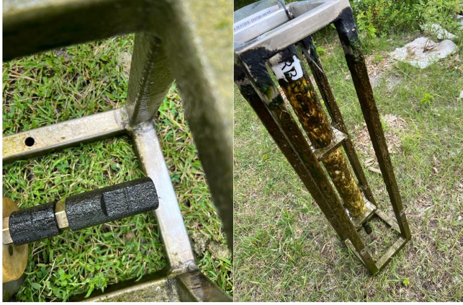
Fig. 7 Algae fouling of turbidity sensor and mounting frame during summer deployment.
