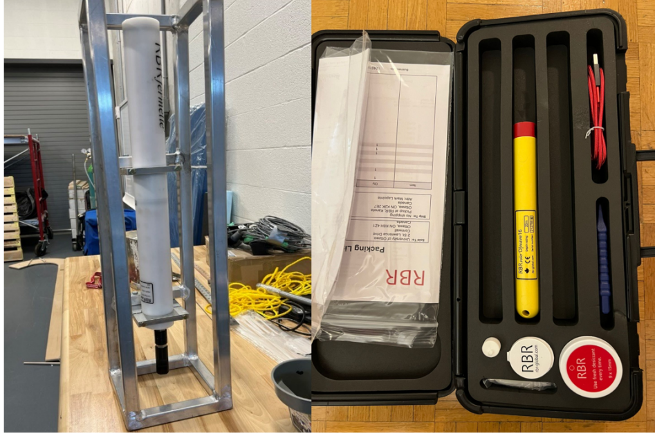
Fig. 3 RBR Duo3 D.TU (left) with 2 Hz turbidity, pressure, and depth sensors; RBR Wave 16 (right) with 16 Hz pressure and depth sampling capabilities.
