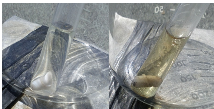
Figure 2.52. Setup of photochemical cyclization reaction. The left image is immediately after initial exposure to sunlight. The right image is after 2.5 hours of exposure to sunlight.
