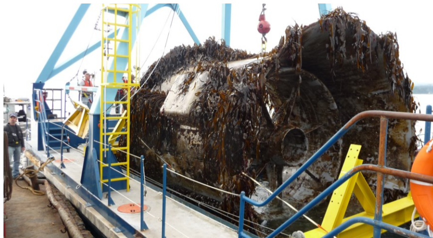
Figure 1.11. Biofouling of Clean Current tidal turbine after 3 years at Race Rocks, BC (source: racerocks.ca )
