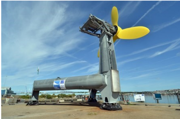
DeltaStream, UK (source: Tidal Energy Ltd.) Horizontal axis
