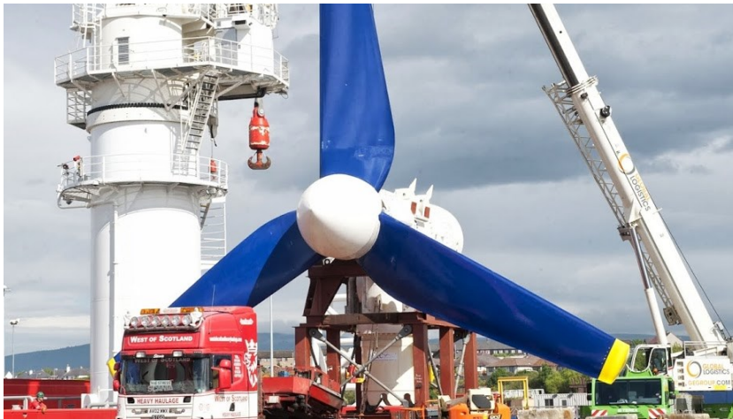
Figure 1.1. Atlantis Resources 1 MW AR1000 tidal turbine (source: Atlantis Resources Ltd.)
