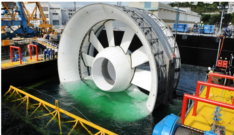
Figure 1.2. OpenHydro 2 MW Open-Centre tidal turbine (source: OpenHydro Group Ltd.)
