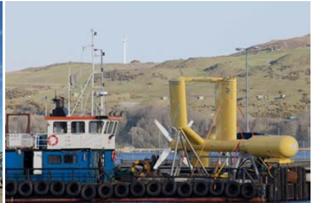
Evopod, UK (source: Oceanflow Energy Ltd.) Horizontal axis. Floating structure.
