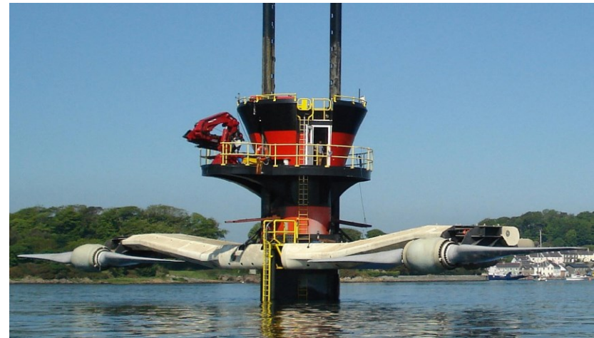
Figure 1.3. Marine Current Turbines 1.2 MW SeaGen tidal turbine (source: Marine Current Turbines Ltd.)
