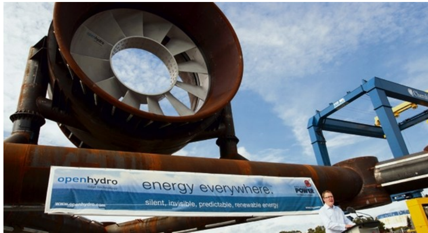
Figure 1.10. OpenHydro 1 MW tidal turbine deployed in the Bay of Fundy (source: OpenHydro Group Ltd.)
