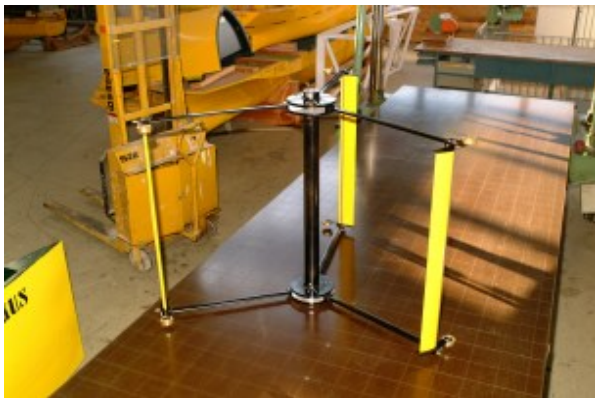
Kobold, Italy (source: Ponte di Archimede) Vertical axis. Floating structure.
