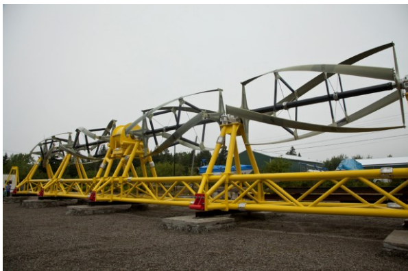
Gorlov Helical Turbine, US (source: GCK Technology Inc.) Vertical axis
