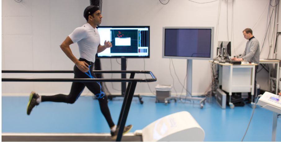
Fig. 1.7: Running analysis solution by Qualisys 6 help improve sports skills and reduce potential injuries with biomechanical data captured by motion technology while a person runs.
