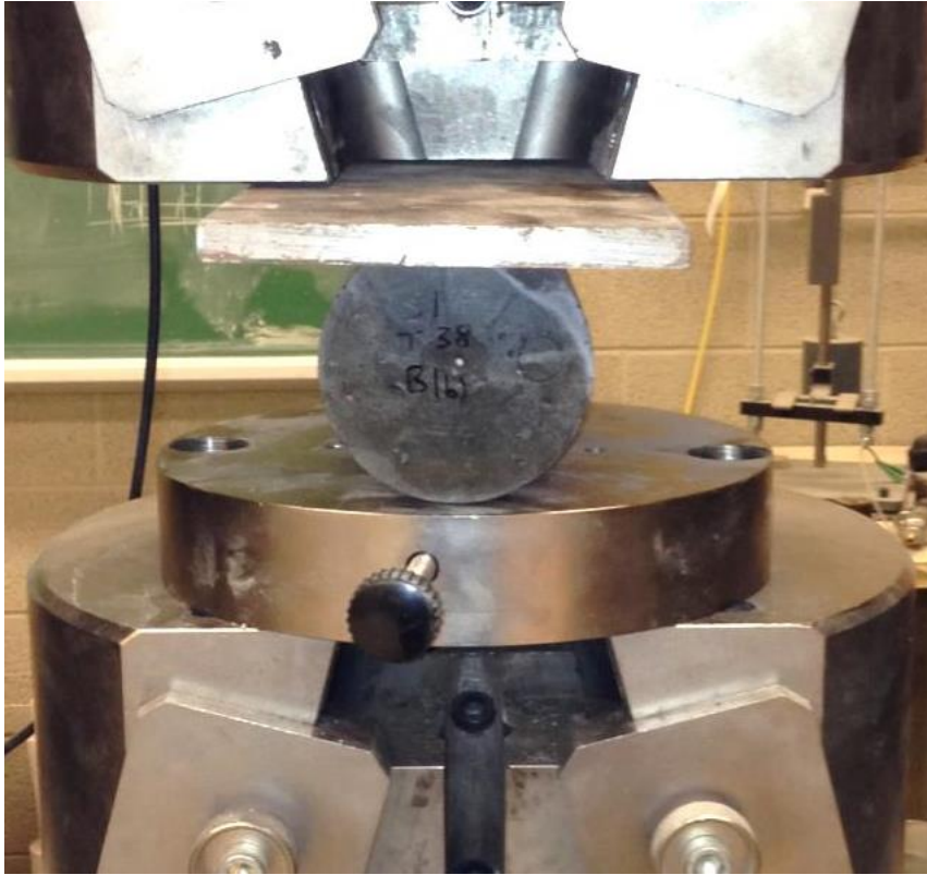
Figure 3.12: Splitting tensile test performed on Galdabini 1890 loading machine
