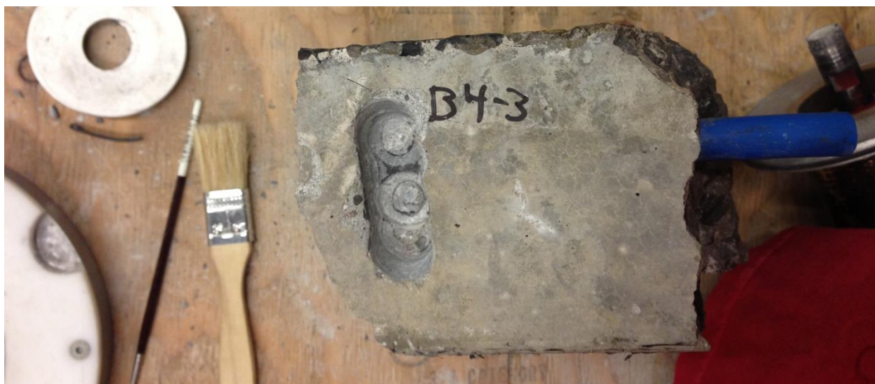
Figure 3.34: Holes created in concrete samples by profile grinder
