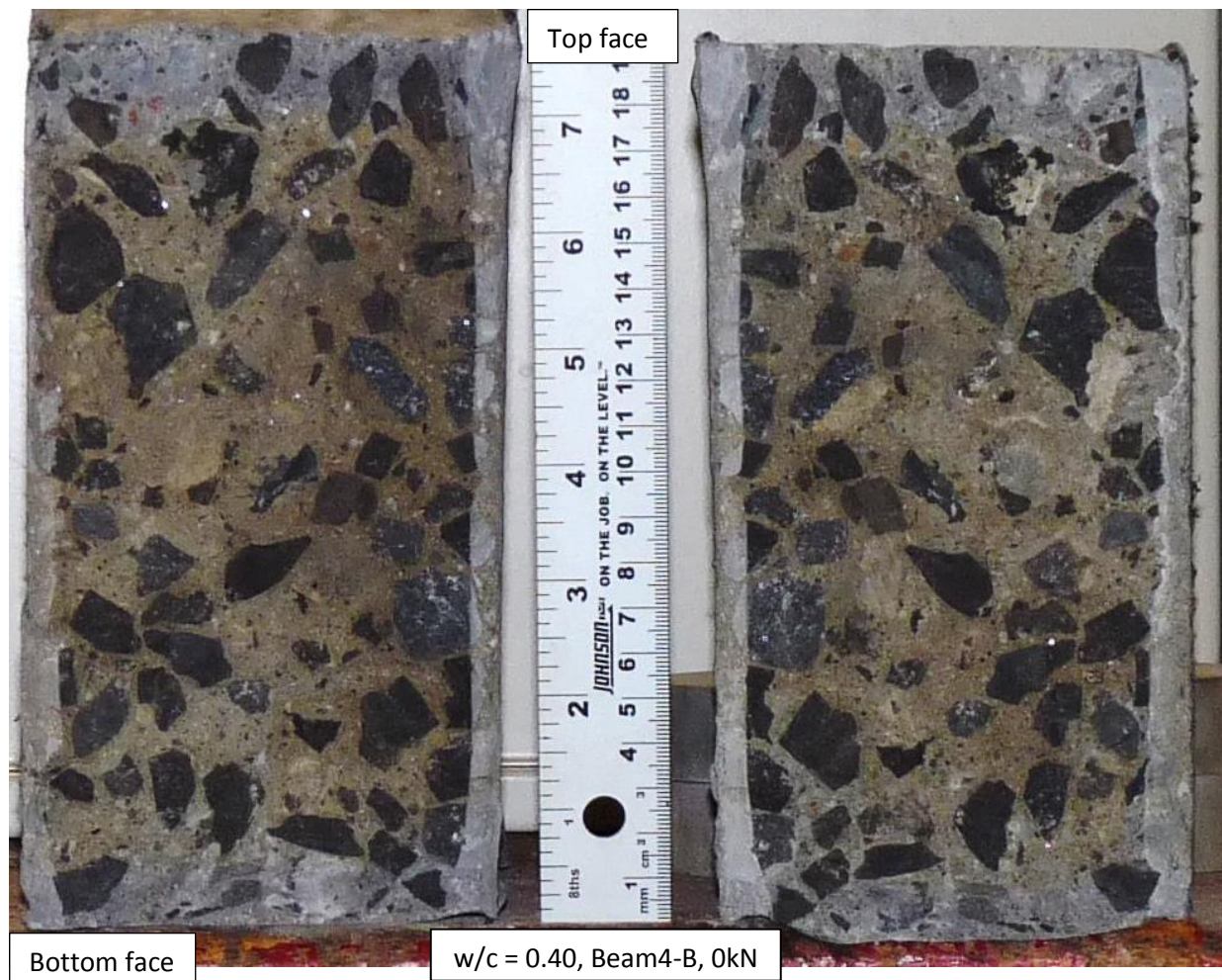
Figure C.14: Chloride penetration depths for beam 4; section B4-B ( w/c = 0.40 , 0 kN)
