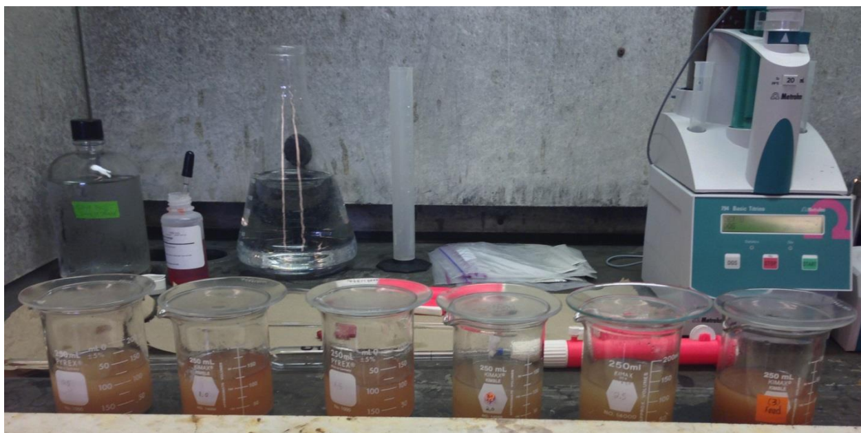
Figure 3.38: Prepared concrete samples digesting and ready to be boiled
