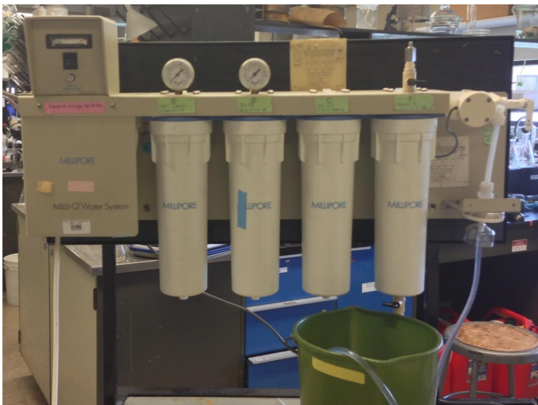
Figure 3.37: Apparatus used to obtain distilled deionized water for sample preparation
