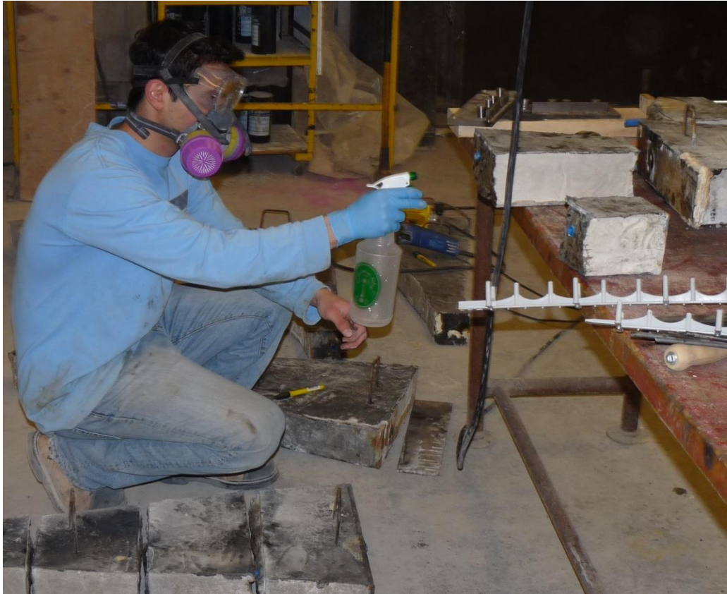
Figure 3.31: Spraying silver nitrate ( \text{AgNO}_3 ) on freshly fractured concrete samples
