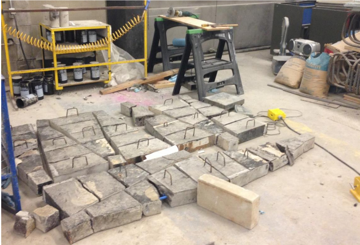
Figure 3.30: All ten concrete beams completely fractured in the lab
