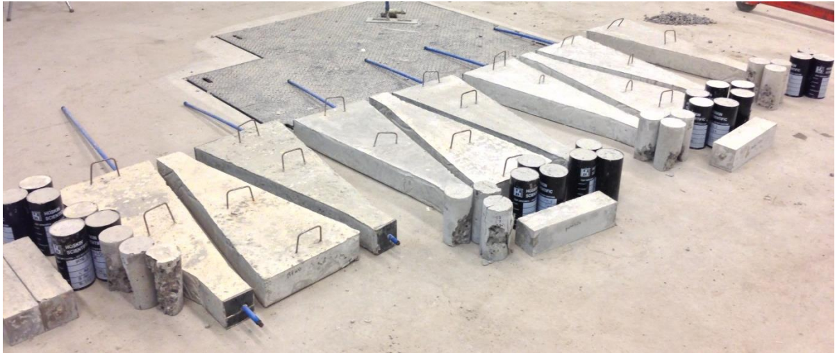
Figure 3.8: Ten concrete beams after curing and prior to post-tensioning, sealing, and material testing
