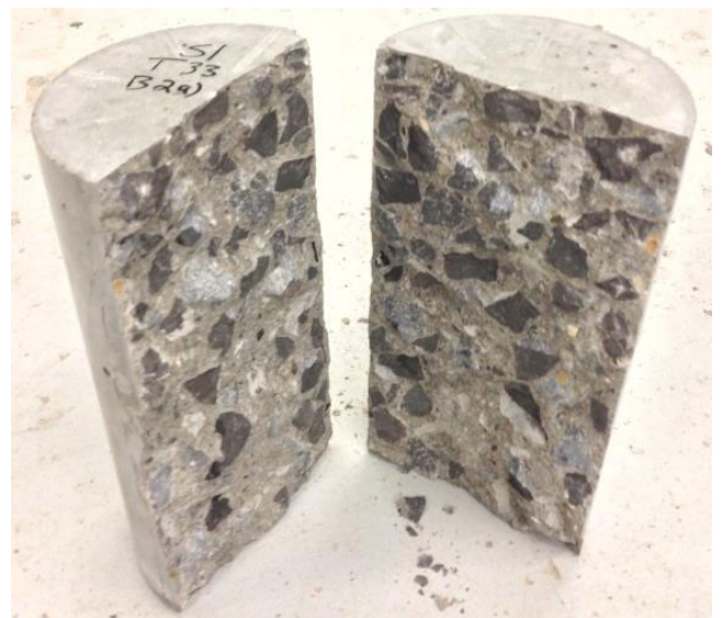
Figure 3.13: Concrete specimens after being failed by splitting tensile test
