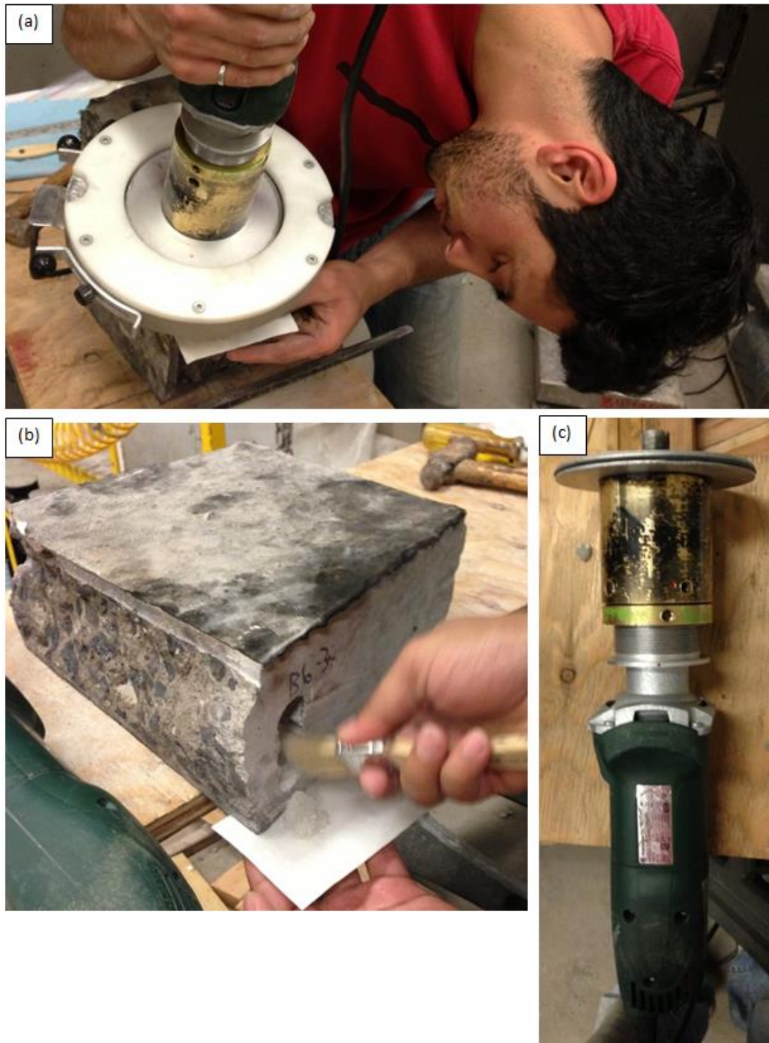
Figure 3.33: Profile grinding process used for each beam section to obtain concrete powder
