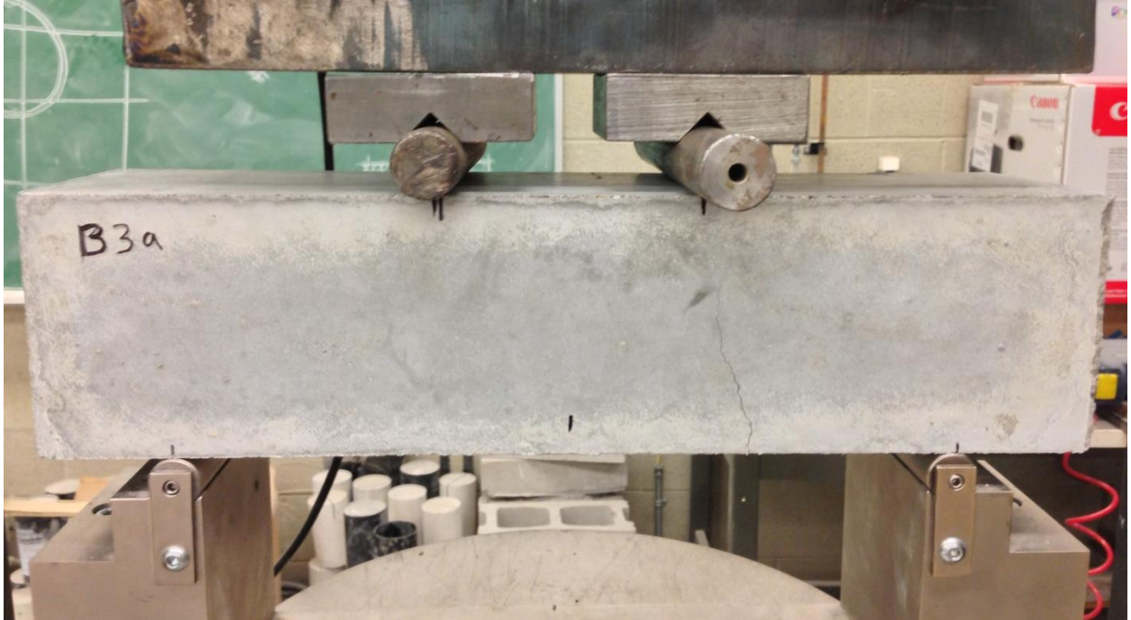
Figure 3.14: Modulus of rupture test being performed on Galdabini 1890 loading machine
