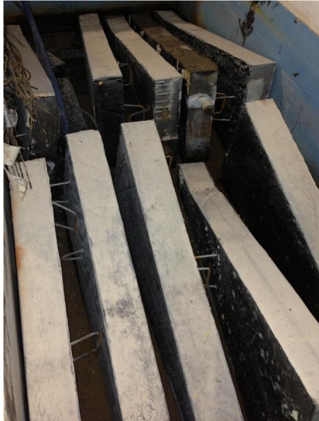
Figure 3.27: Concrete beams drying after 12 weeks of exposure in tank
