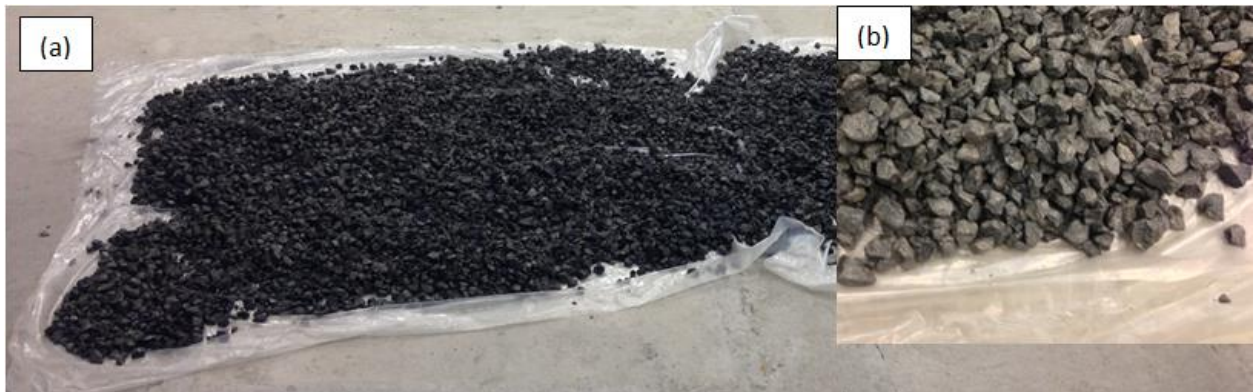
Figure 3.4: (a) Coarse aggregate after washing and (b) After 24 hr of air drying to SSD
