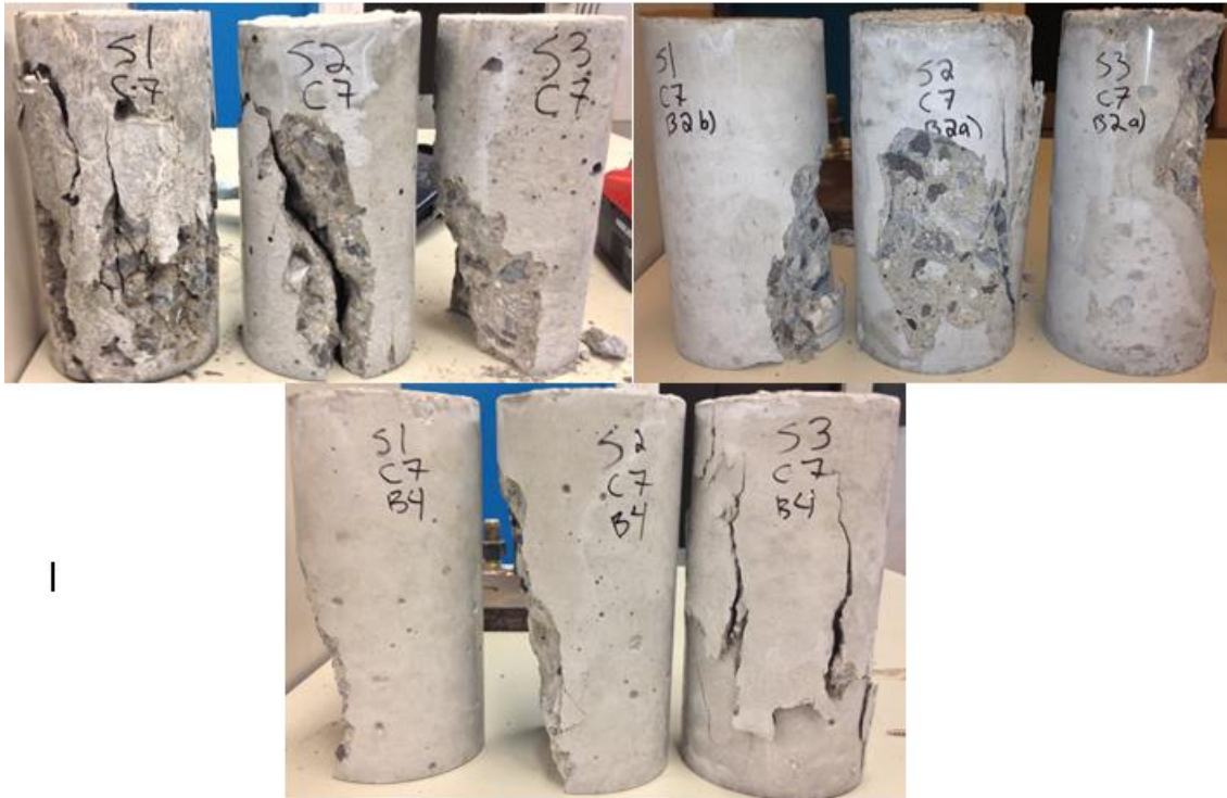
Figure B.1: Failure patterns of cylinders from all batches (7d compression)
