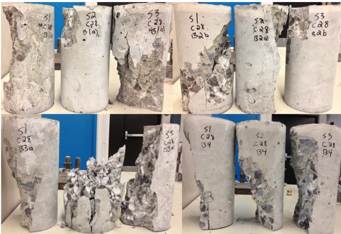
Figure B.2: Failure patterns of cylinders from all batches (28d compression)
