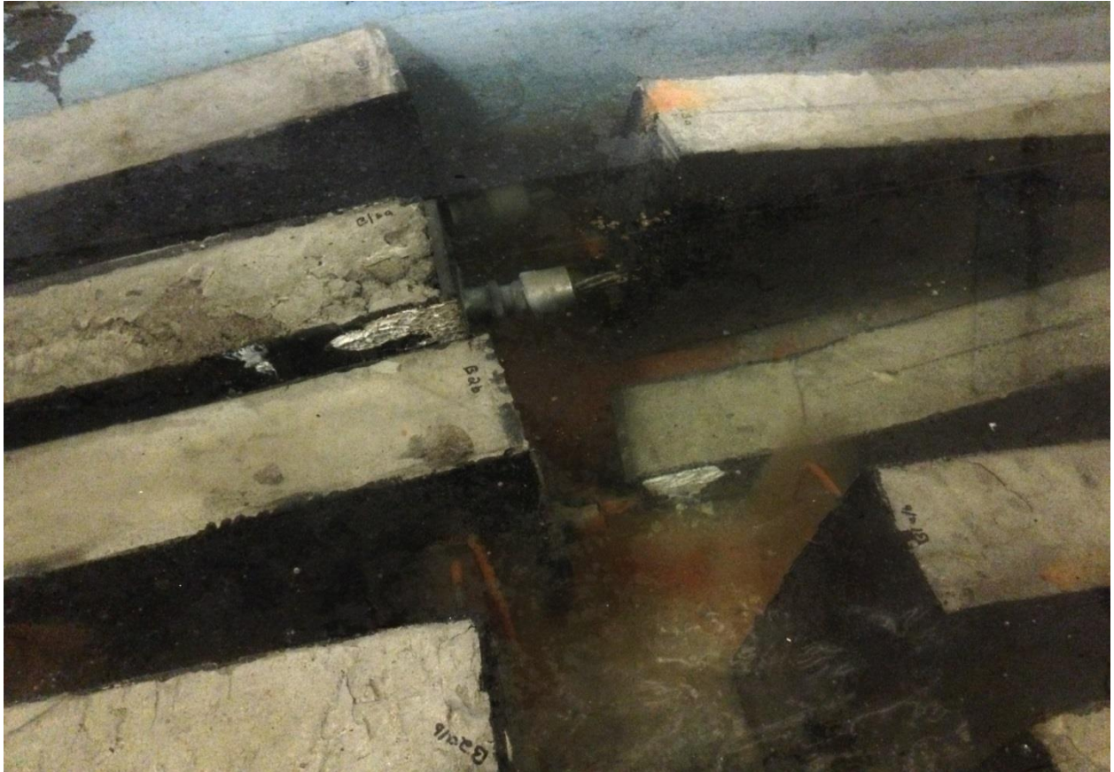
Figure 3.26: Submerged concrete specimens after one month exposure time
