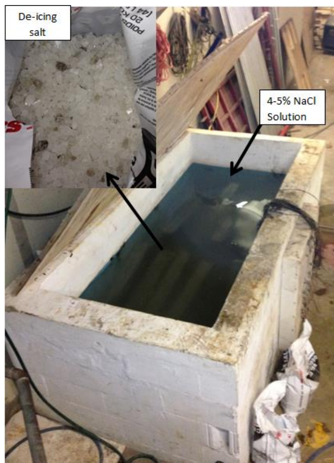
Figure 3.23: Immersion of concrete beams into 4-5% NaCl solution
