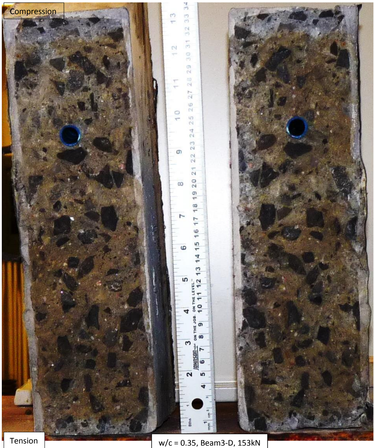
Figure C.12: Chloride penetration depths for beam 3; section B3-D ( w/c = 0.35 , 153 kN)
