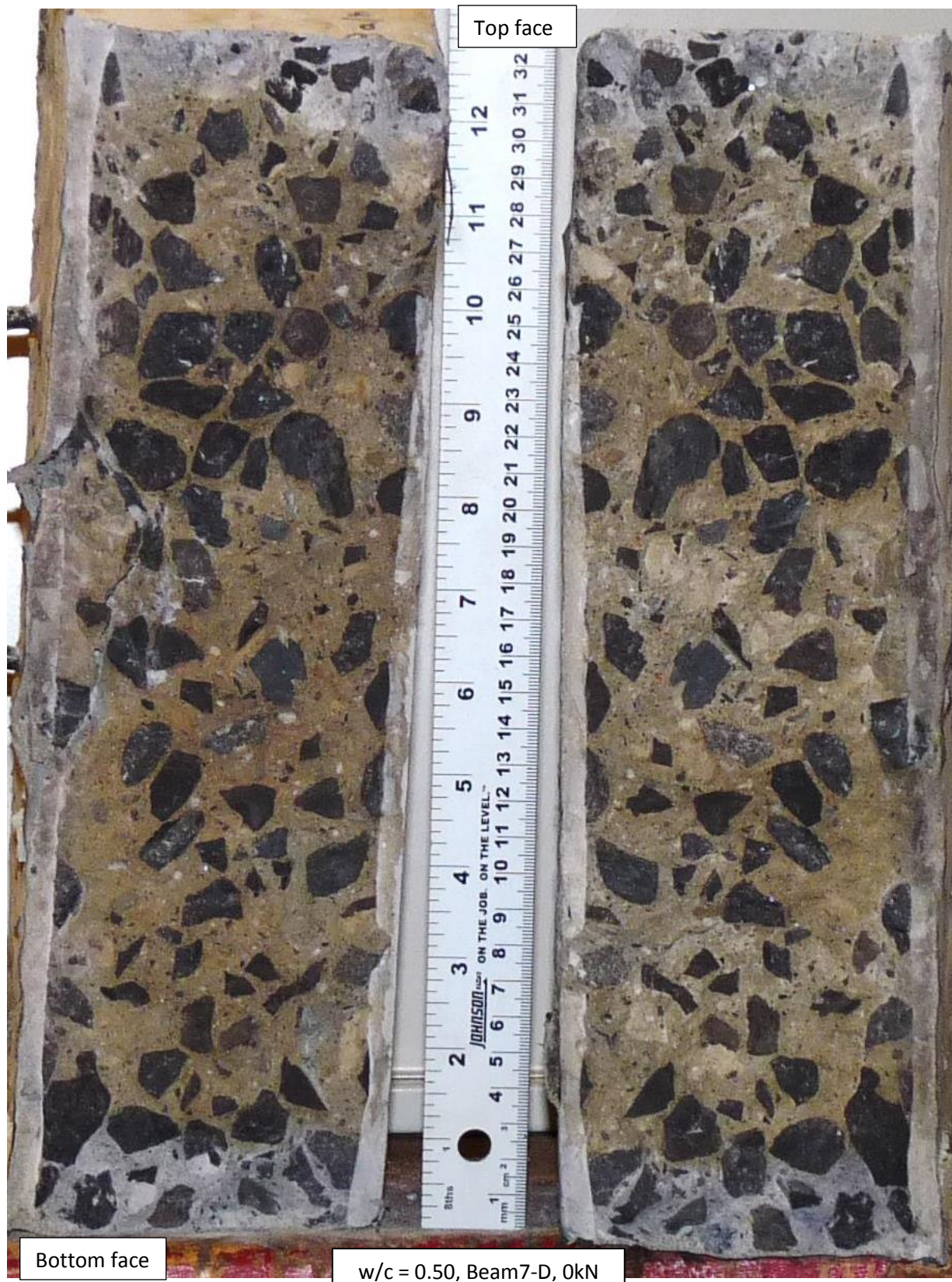
Figure C.28: Chloride penetration depths for beam 7; section B7-D ( w/c = 0.50 , 0 kN)
