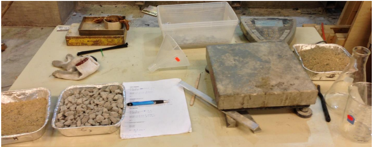
Figure 3.3: Determining absorption and moisture contents of aggregates in the lab
