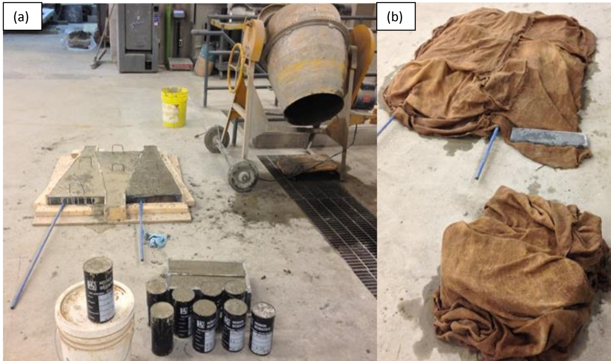
Figure 3.7: (a) Formwork after casting and levelling (b) Concrete being burlap cured in the lab
