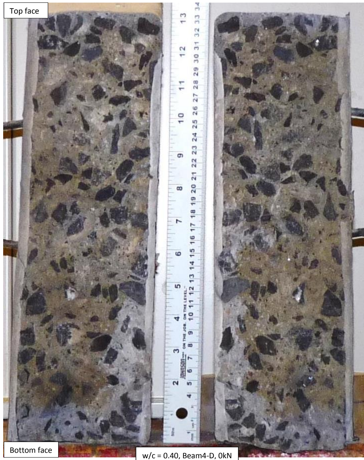
Figure C.16: Chloride penetration depths for beam 4; section B4-D ( w/c = 0.40 , 0 kN)
