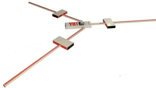
Figure A.2: The Y-Balance Test kit, displaying the central platform with three reaching arms/reach indicator used to measure multidirectional reach distances.
