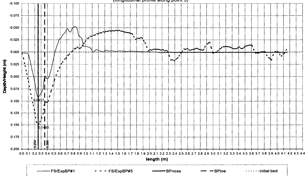
Scour depths and erosion/deposition features around bridge pier in FS (longitudinal profile along point 5)
