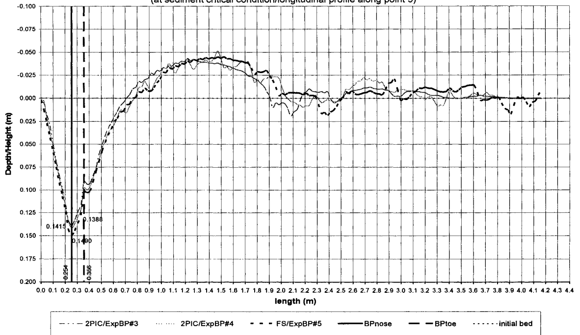
Scour depths and erosion/deposition features around bridge pier in FS and 2PIC (at sediment critical condition/longitudinal profile along point 5)
