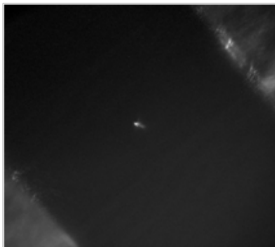
Figure 4.3: The ^{88}\text{Sr}^+ ion fluorescence seen with camera in endcap trap (photo courtesy of P. Dubé).
