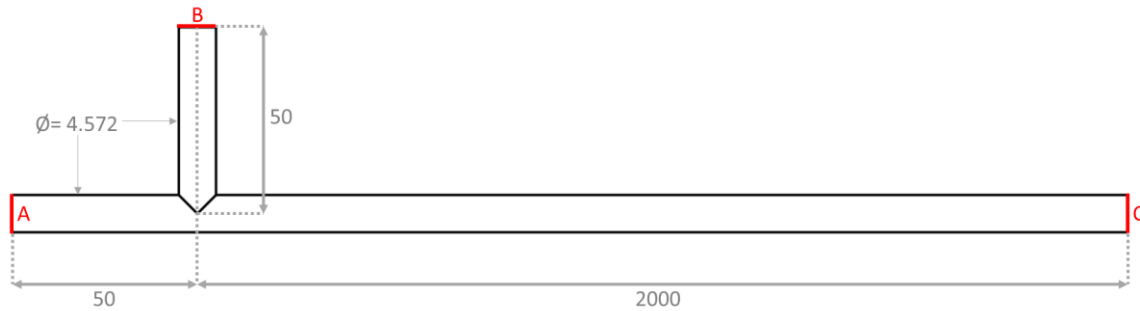
Figure 20: A 2D representation of the 3D computational domain dimensions for the powder preheater model. Red shows inlets and outlets. Not to scale. All dimensions in mm.
