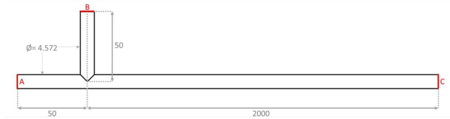
Figure 6. Schematic of the 3D computational domain dimensions for the powder preheater model. Red shows inlets and outlets. Not to scale. All dimensions in mm.
