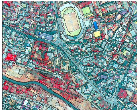
Figure 60: Classification of an urban area using object-based image analysis. Object based image analysis by Uddinkabir, Wikimedia Commons, CC BY-SA 4.0.
