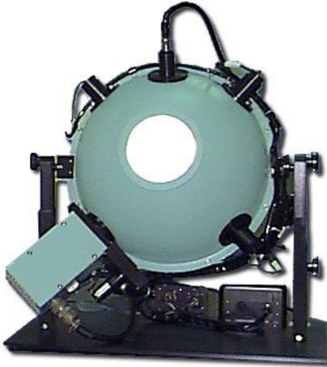
Figure 18: Integrating sphere used for sensor calibration. Commercial Integrating Sphere by Electro Optical Industries, Wikimedia Commons, CC BY-SA 3.0.
