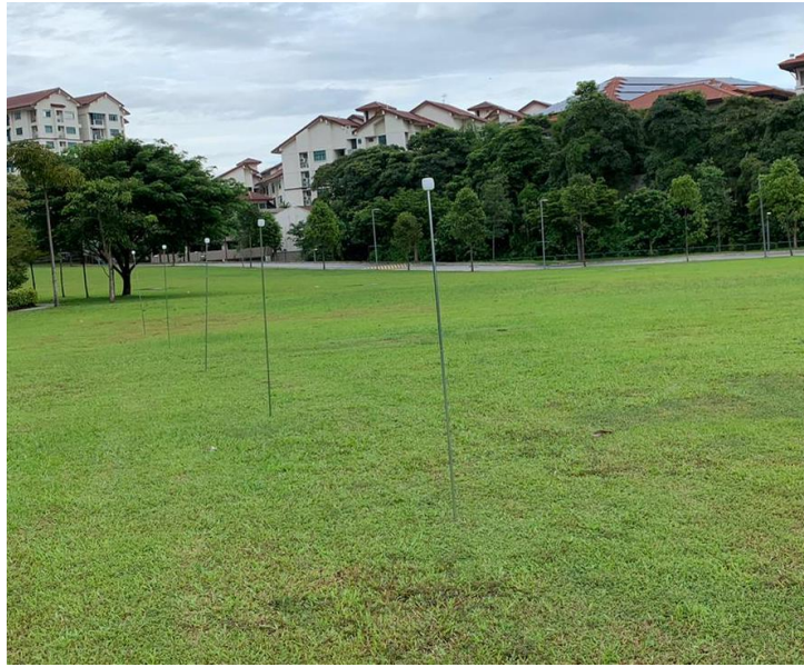
Figure 3.10: Experimental set-up of Beacon signal range test. In an open ground, each beacon is mounted on a pole and placed at 1 meter interval from each other for the first 5 meters (5 beacons), and the interval is increased to 5 meters for the next 45 meters (10 beacons). The first beacon is placed 0.5 meter from the mobile and the last beacon at 50.5 meters
