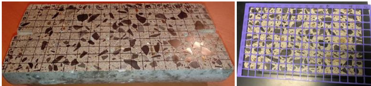
Figure 2-7 - (a) A well-polished, highly reflective surface featuring a grid, with visible light reflection in the bottom-right corner (b) a 3D-printed grid positioned over the polished surface, adapted from Sanchez, (2024)
