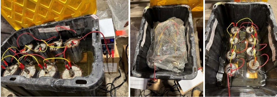
Figure 3-9 - Accelerated corrosion setup: concrete specimens in NaCl solution connected to the power supply
