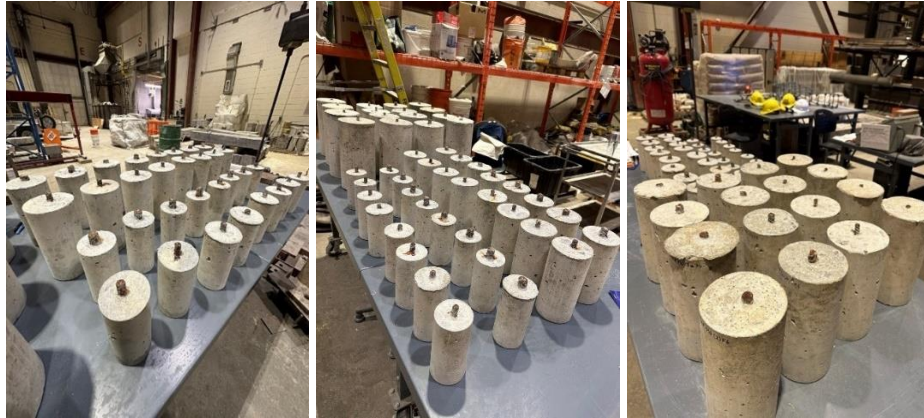
Figure 3-3 - Concrete specimens after 28 days of curing, ready for accelerated corrosion test
