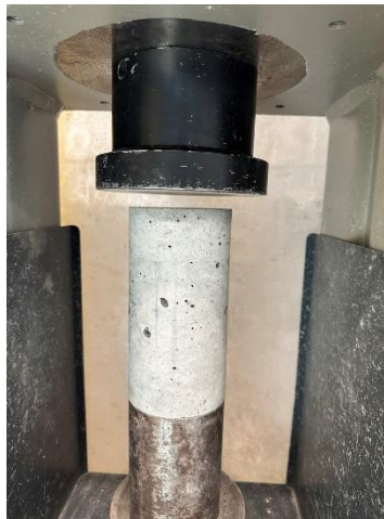
Figure 3-4 - Concrete specimens during compressive strength test
