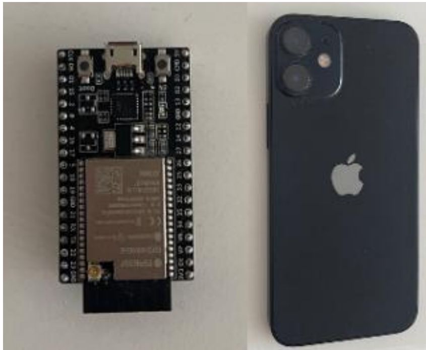
Figure 20 Feasibility study 2 - system instruments: iPhone 12 mini (right) as a WiFi receiver and ESP32 (left) as a WiFi transceiver.
