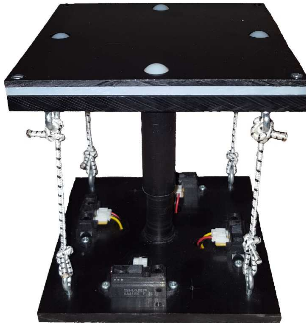
Figure 4.13 : Rolling Contacting Layer Mounted onto Compliant Wrist
