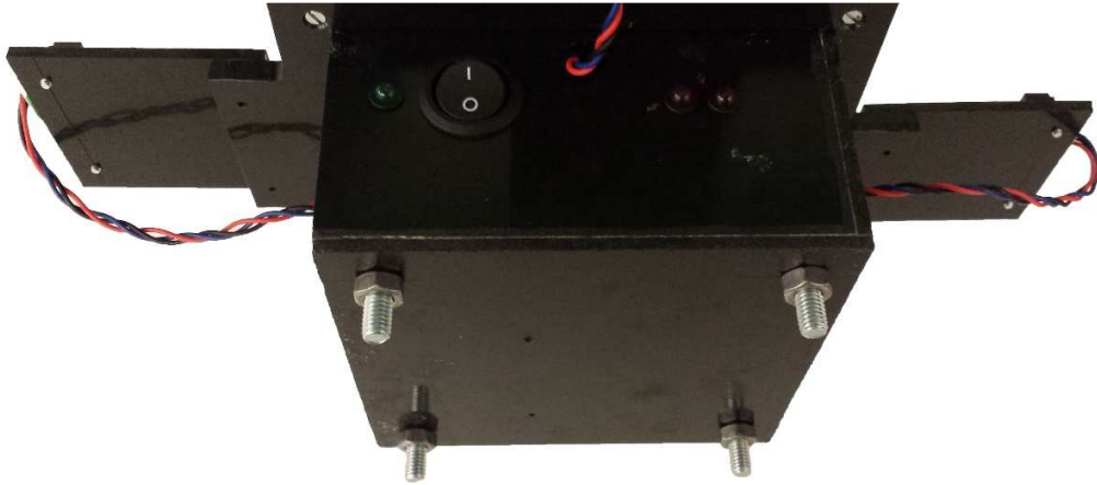
Figure 4.14 : Bottom of Electronics Enclosure showing Mounting Bolts and Nuts
