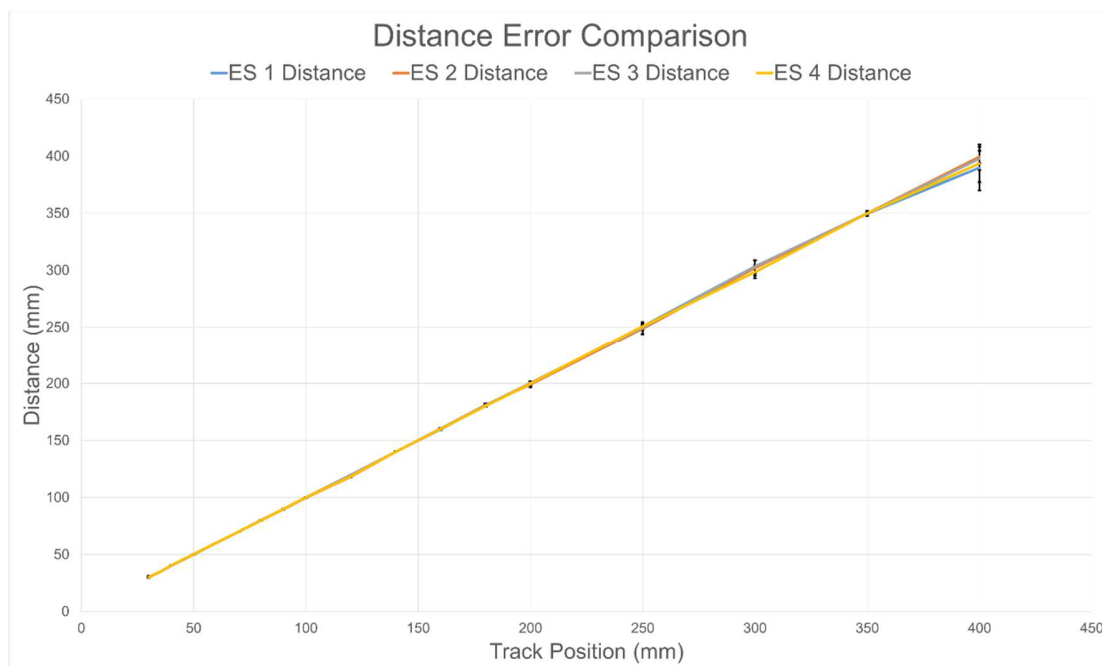
Figure 6.14 : Comparison of Calibrated Sensor Distance Response Curves
