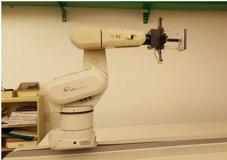
Figure 6.37 : Compliant Wrist Mounted on the CRS-F3 Manipulator to Act as its End-Effector
