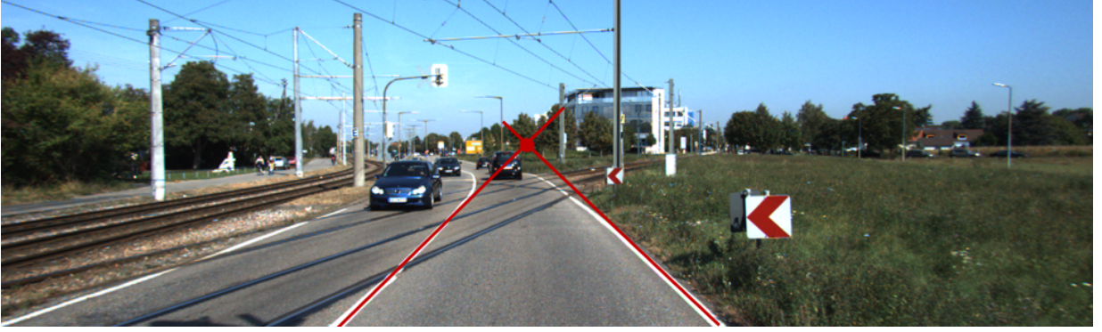
Figure 2.34: The vanishing point in the current frame.
