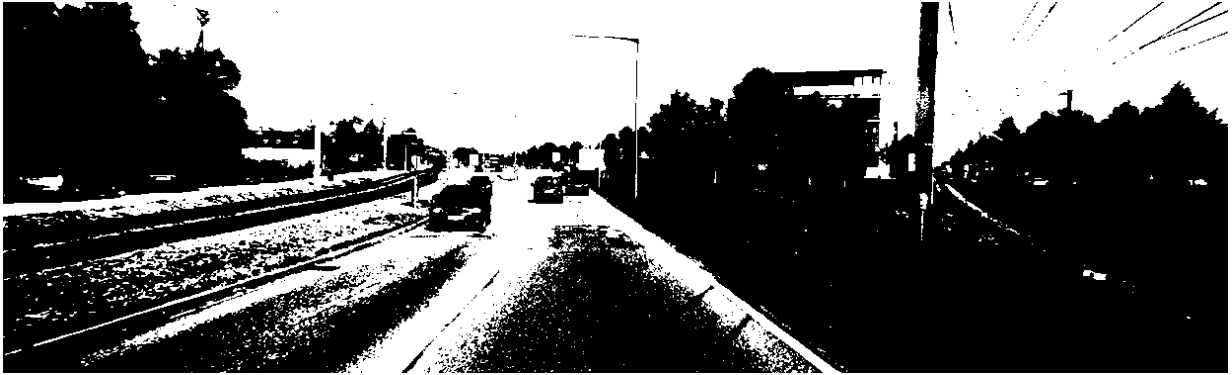
Figure 2.8: The result of setting threshold as 128.
