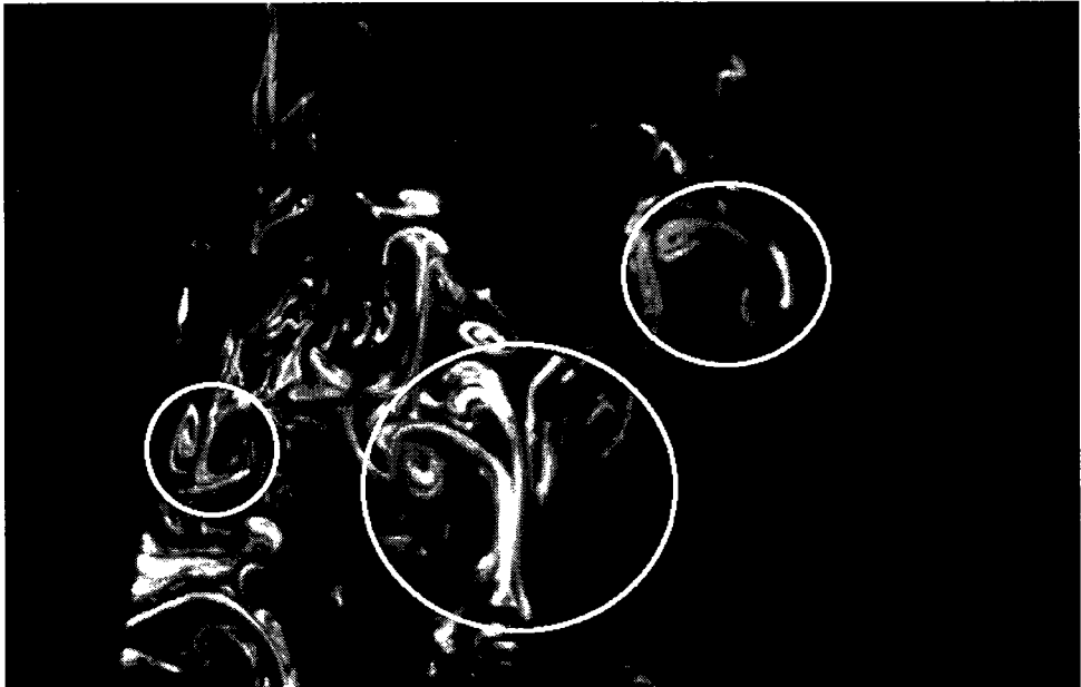
Figure 2.7: Dye visualisation of mushroom-shaped vortex pairs in an inclined plane 45^\circ between the x_1 - x_3 and x_2 - x_3 planes. (Reproduced from [23]).
