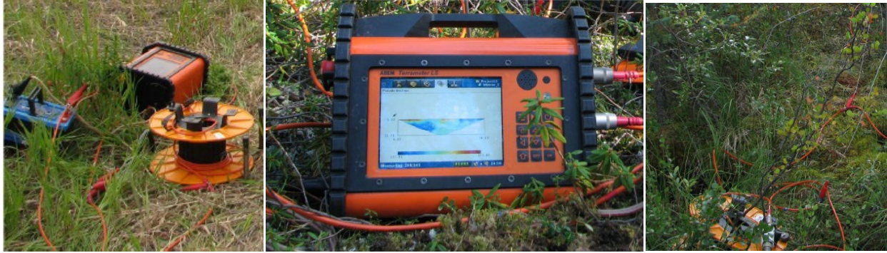
Figure 9: ABEM Terrameter LS being used in the field to complete electrical resistivity tomography surveys (Lewkowicz et al. 2013)
