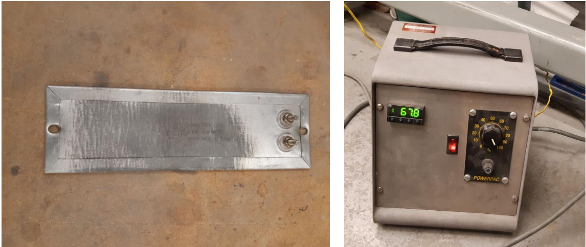
Figure 4.16. Strip heater (left) and potentiometer (right).
