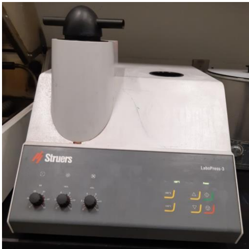
Figure 4.20. Struers LaboPress-3 mounting machine (left) and MultiFast Red resin (right).
