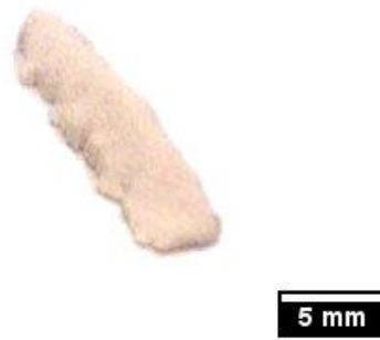
Figure 5.2. Delaminated trail of pure PEEK from a grit-blasted substrate (400°C, 2.07 MPa, 2 mm/s).
