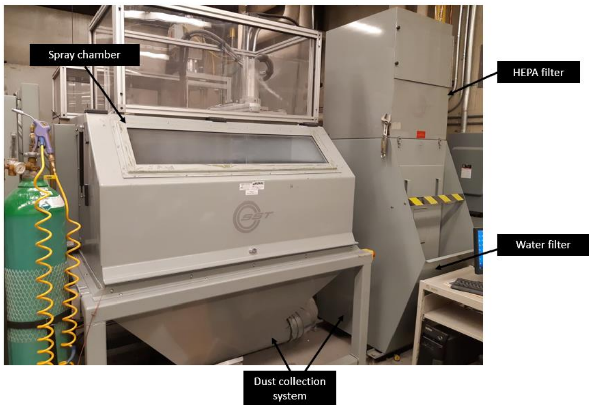
Figure 4.14. CGDS spray chamber and dust collection system.
