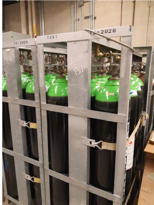
Figure 4.15. Nitrogen bottle packs used in the CGDS process.
