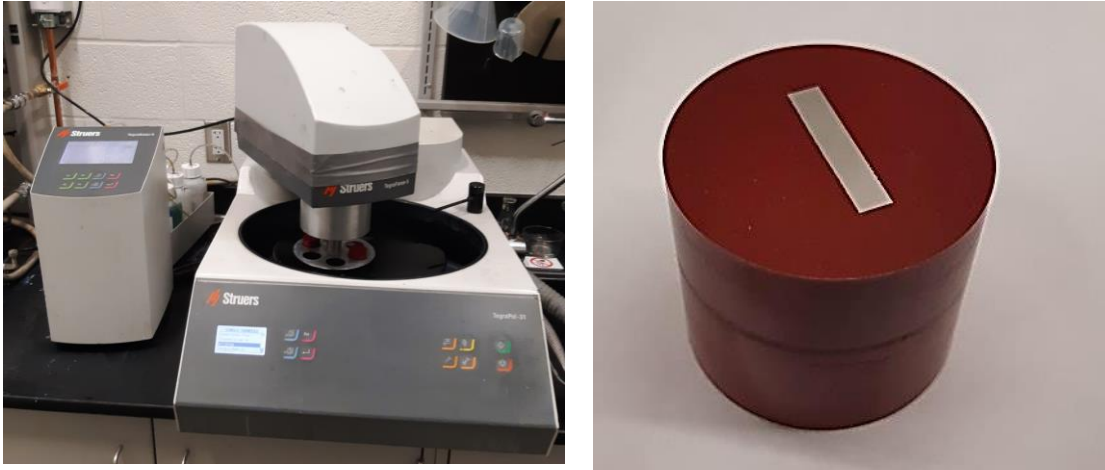
Figure 4.21. Struers TegraPol-31 polishing machine (left) and mounted/polished sample.
