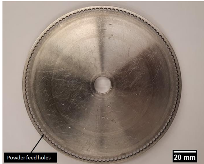
Figure 4.12. Large hole powder feeder wheel with 120 holes.
