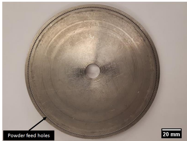
Figure 4.13. Medium hole powder feeder wheel with 240 holes.
