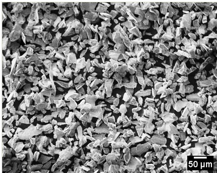
Figure 4.3. SEM image of the SST-G0001 alumina powder.
