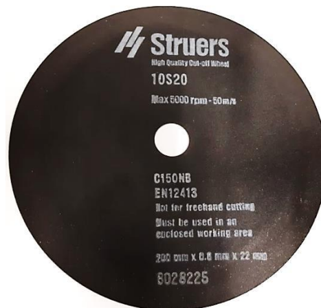
Figure 4.18. Cut-off wheel used with the Struer Secotom-10 cutting machine.
