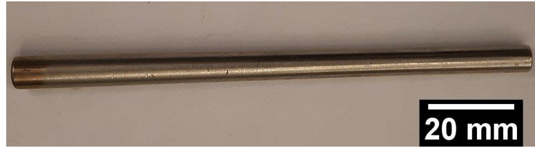
Figure 4.9. Centerline (Windsor) Ltd. Stainless steel nozzle.
