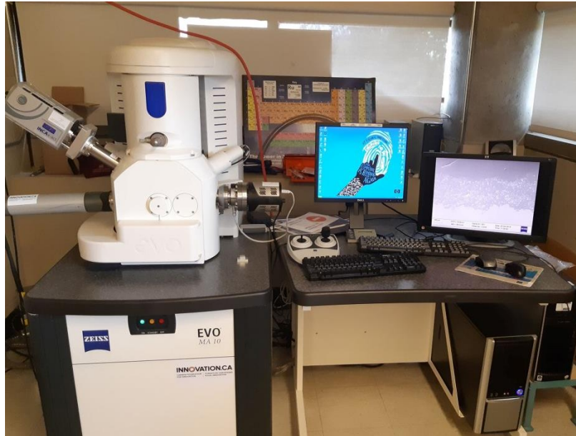
Figure 4.23. Scanning electron microscope (EVO-MA10, Zeiss, UK).
