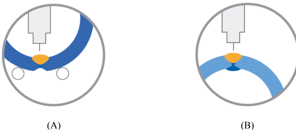
Figure 1. 4 (A) Inside and (B) Outside seam welding of the formed pipe (from EUROPIPE GmbH)
