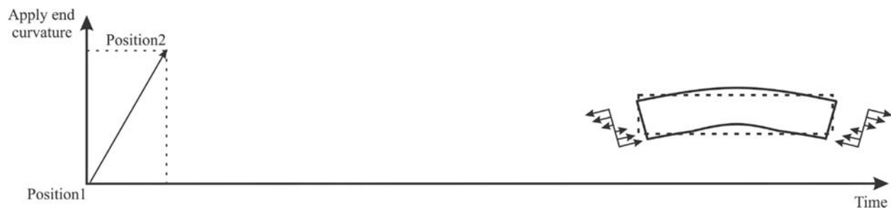
Figure 5. 1 Loading path for P00S specimen subjected to pure end moments
