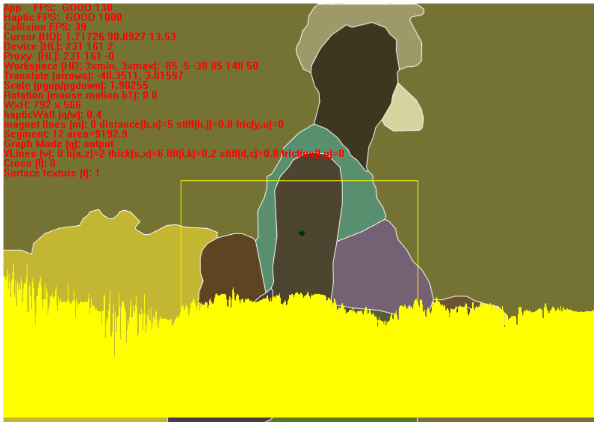
Figure 3.8: Our haptic image exploration system running in debug mode. In this mode, the image is rendered visually as well as haptically. The yellow graph shows the amplitude of the force feedback output. The red text displays the frame per second of each threads, the cursor position before and after transformation, the proxy position, the workspace limits, the current translation and scaling amount and the status and parameters for various features supported by our system. The yellow lines delimit the haptic workspace.
