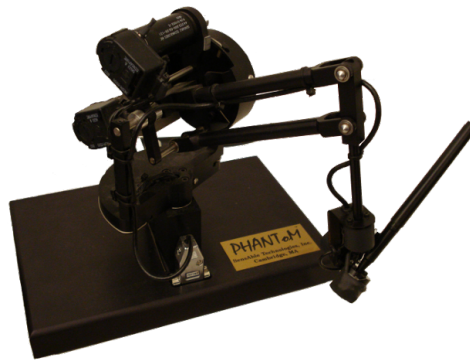
Figure 1.1: PHANTOM 1.0 point contact device by SensAble Technology.
