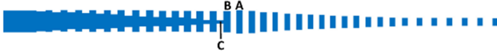
Figure 3.7: Geometry of a subwavelength edge coupler, where section A denotes the grating width at the end of the taper from the tip of the edge coupler, B denotes the starting grating width of the following taper section, and C denotes the starting width of the solid core waveguide taper which couples the mode to a single-mode waveguide. Figure from [117].
