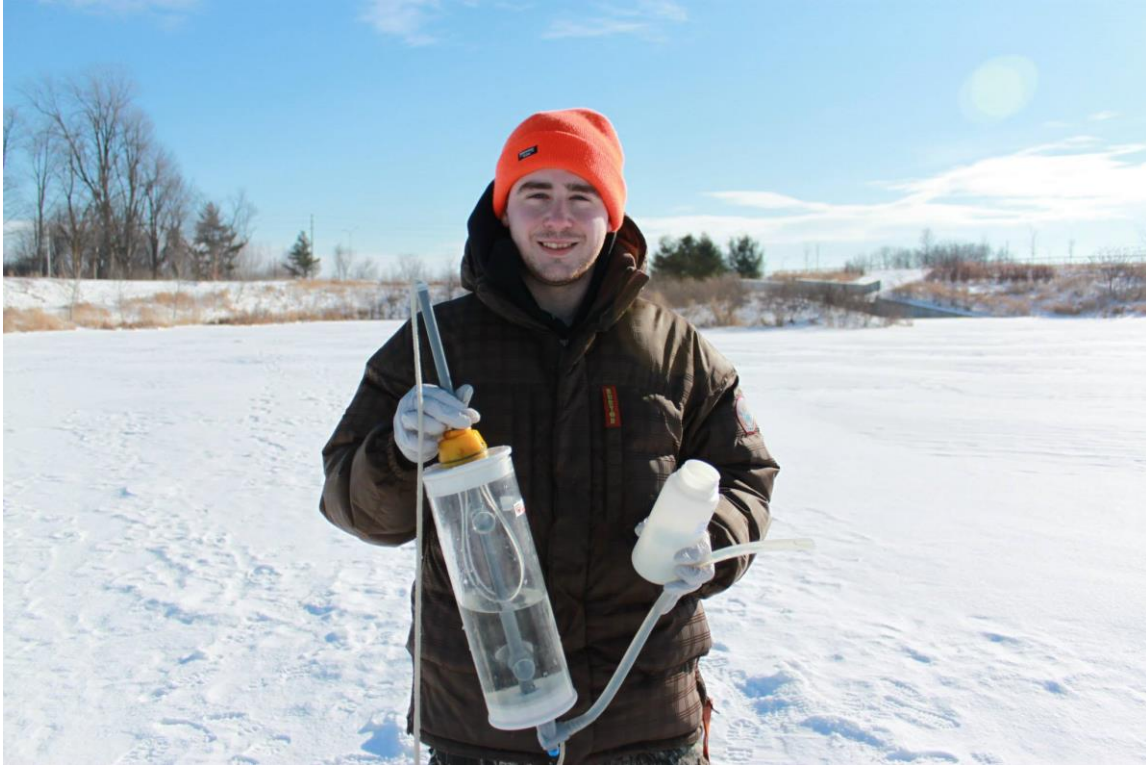
Figure 3.2 Collection of water samples in winter, with the modified hose attachment installed on the water sampler
