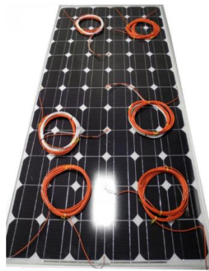
Fig. 3.11. The solar panel and sensors (Mehranfar, 2014)
