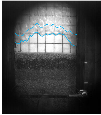
Figure 29: Video Snapshot for Exact Method of Bore Front Tracking
