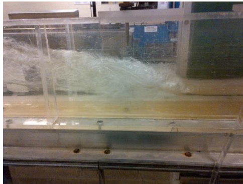
Figure 4: Hydraulic Jump in a Laboratory
