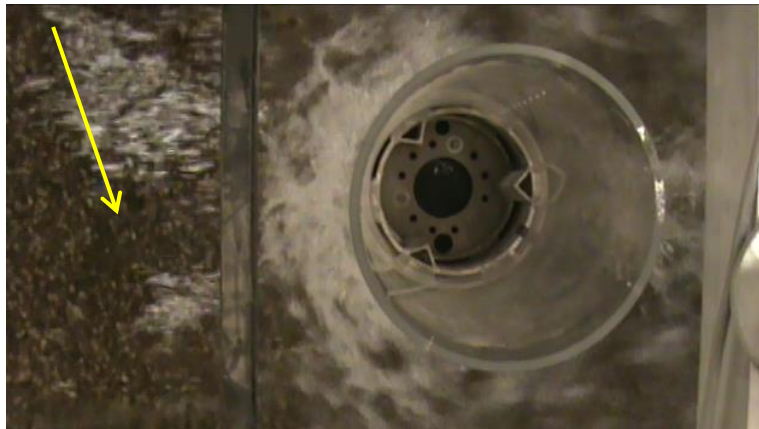
Figure 45: Gravel Particle Movement as Bedload (Test 5, 11 sec.)
