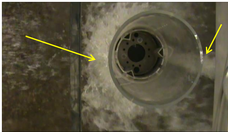
Figure 41: Initial Bore Impact on Structure (Test 5, 8 sec.)
