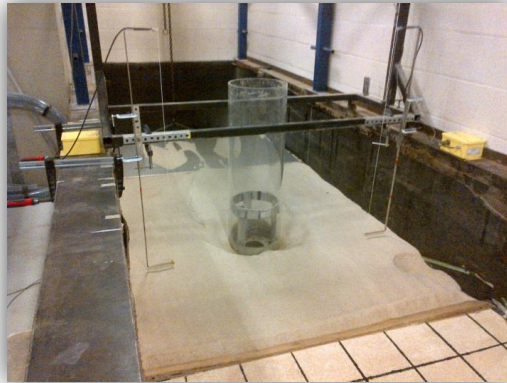
Figure 24: Left: Two Wave Gauges at Structure, Right: Wave Gauge in Reservoir behind Swinging Gate
