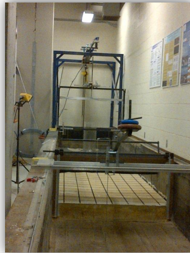
Figure 24: Left: Two Wave Gauges at Structure, Right: Wave Gauge in Reservoir behind Swinging Gate
