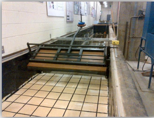
Figure 22: Left: Wood and Steel Framed Swinging Gate, Right: Wave Absorber
