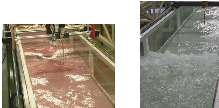
Figure 6: Undular Bore and Fully Developed Bore (Koch & Chanson, 2009)
