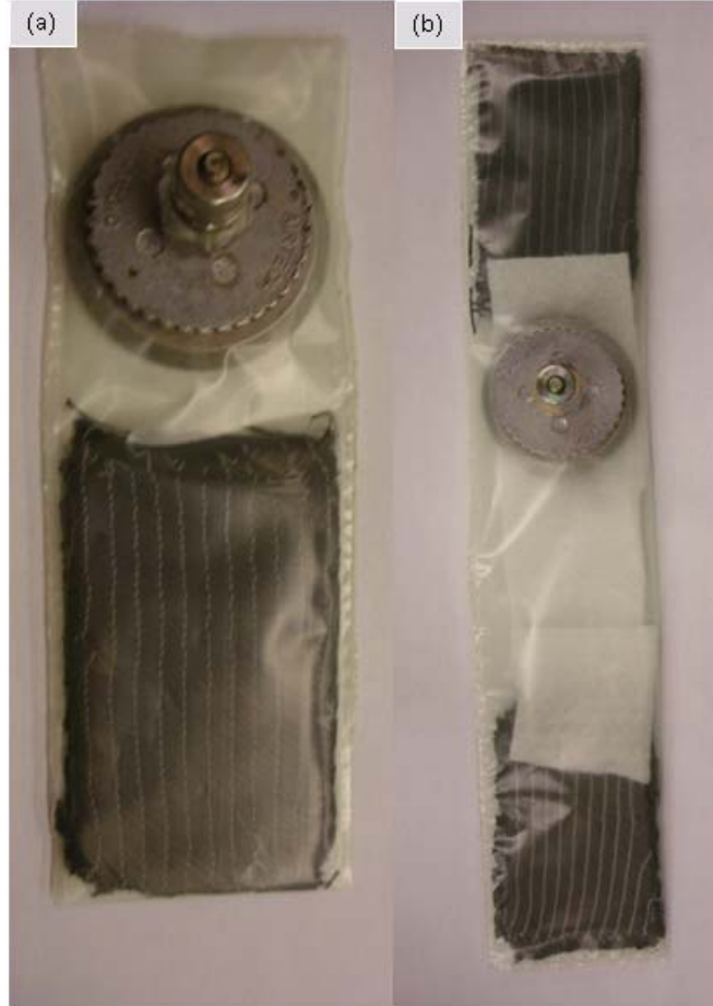
Figure 3.5 - Vacuumed samples for (a) in-plane and (b) through-thickness thermal conductivity measurements of the non-crimp fabric
