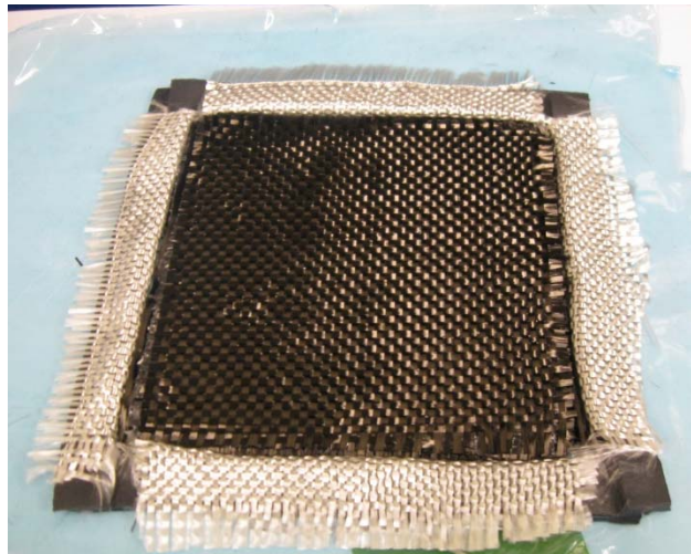
Figure 4.10 - Vacuum bag sealant tape wrapped with fibreglass around layup: plate P10 (d)
