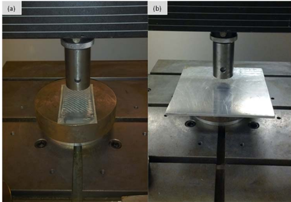
Figure 3.7 - Compaction setup on Instron 4482 universal testing frame: (a) sample placed on bottom fixture (b) aluminium platen placed on top of sample
