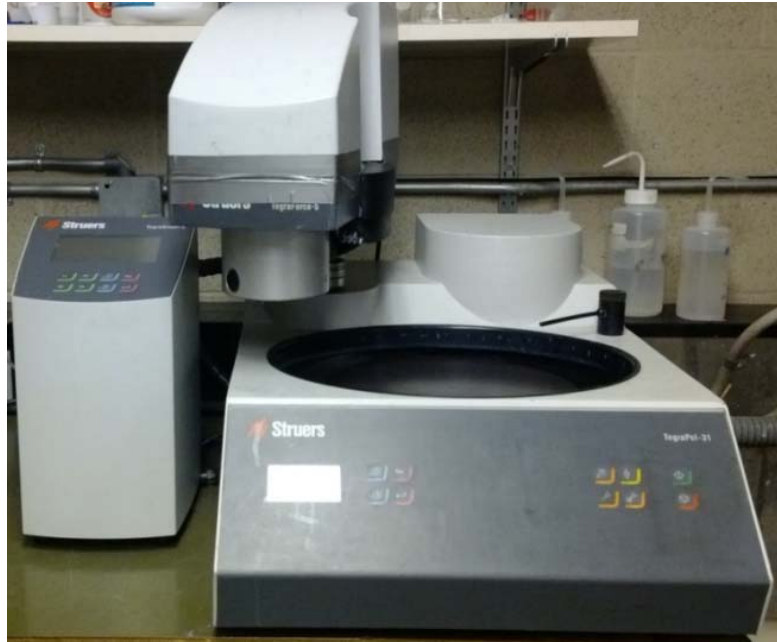
Figure 4.18 - TegraPol-31 polishing system
