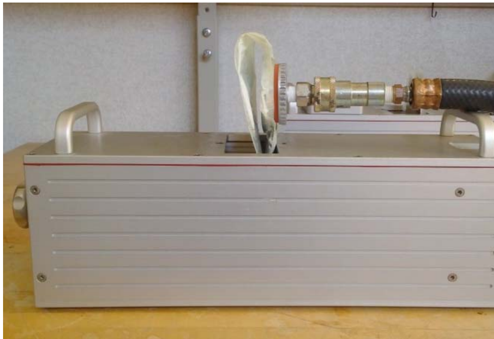
Figure 3.9 - Through-thickness thermal conductivity measurement of non-crimp fabric sample in THASYS
