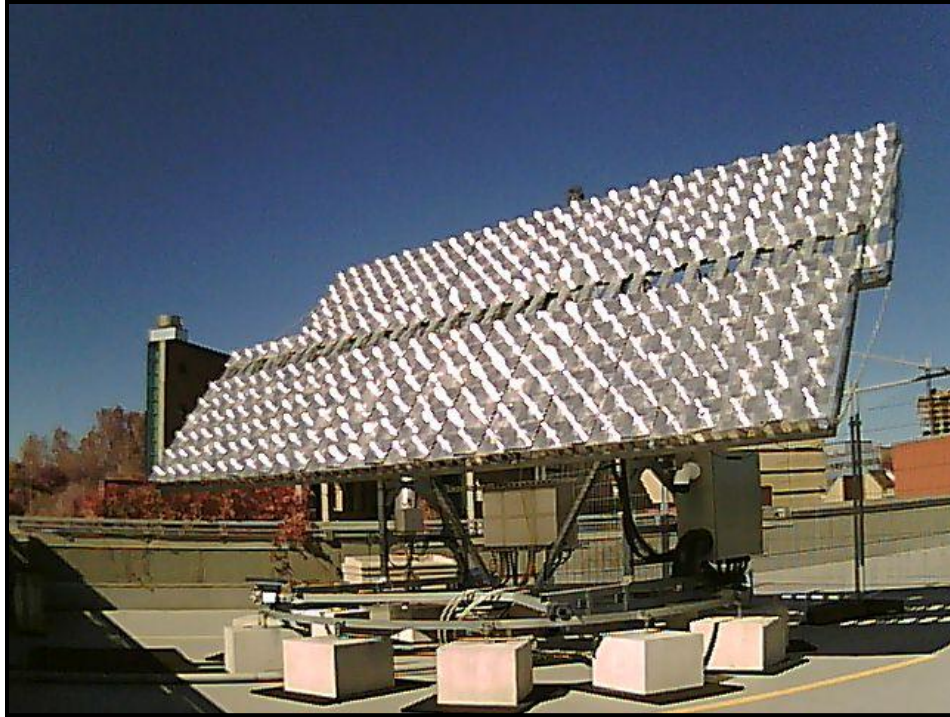
Figure 1-17: The APECS demonstrator May 9 th , 2011. The APECS demonstrator holds high-efficiency triple-junction solar cells that have been integrated into Morgan Solar concentrating optics that are pointed at the sun with a Golden Sun dual axis tracker.
