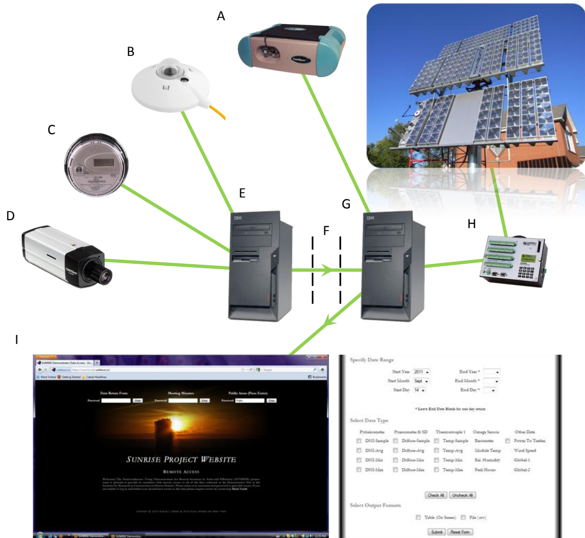
Figure 3-1: Schematic of the SUNRISE demonstrator remote data acquisition system.
