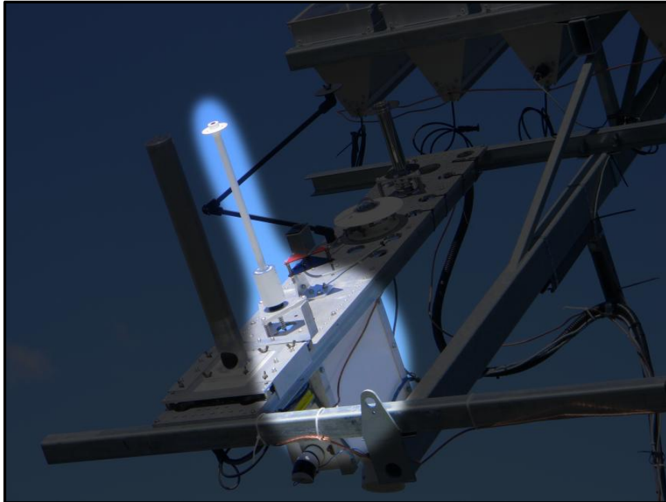
Figure 3-12: The highlighted instrument is the spectroradiometer mounted on the SUNRISE demonstrator in a ventilated heated enclosure. The custom enclosure allows the instrument to be left outdoors to collect spectra continuously even through a harsh Canadian winter. The direct attachment (white tube pointing at the sun) ensures that only the direct component of the insolation reached the diffuse cosine receptor which couples the light into the spectrometers fiber input.
