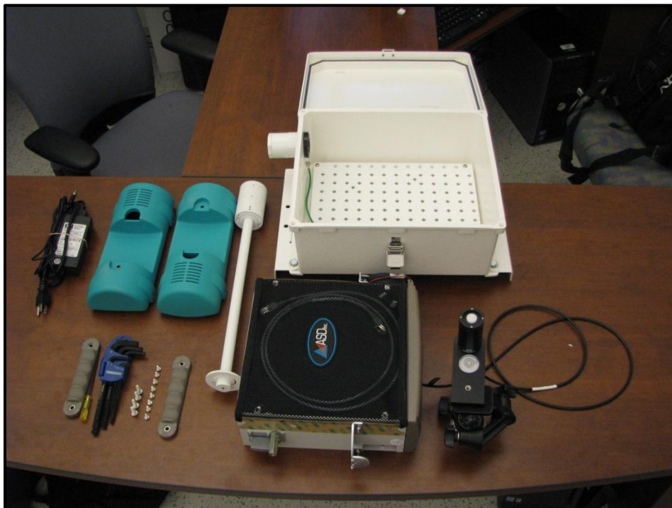
Figure 3-13: ASD Inc. Field Spectrometer configured as a spectroradiometer sitting beside the enclosure that was retrofit to keep the instrument cool in the summer and warm in the winter.
