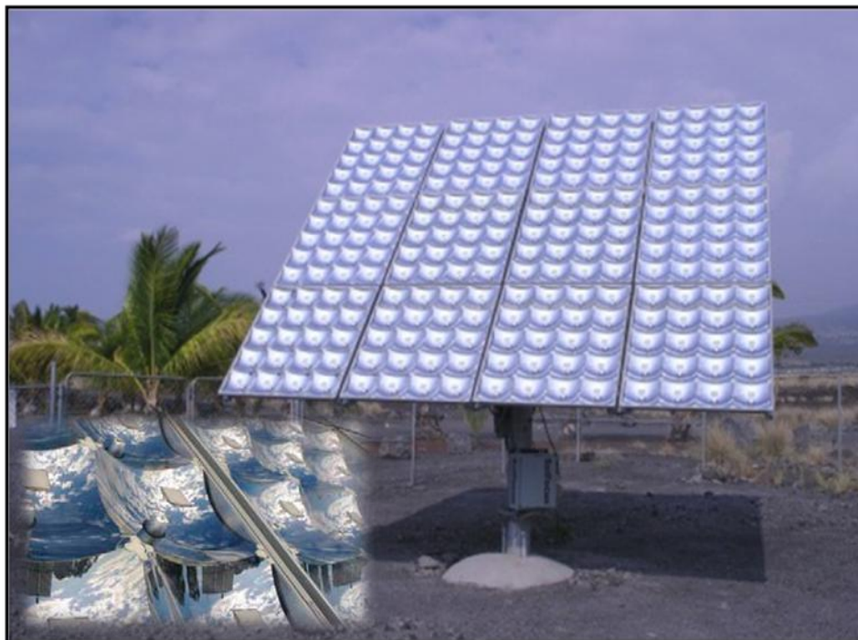
Figure 1-19: SolFocus two stage reflective optics. This demonstrator system was deployed in Kailua Kona at the National Energy Laboratory of Hawaii [31].
