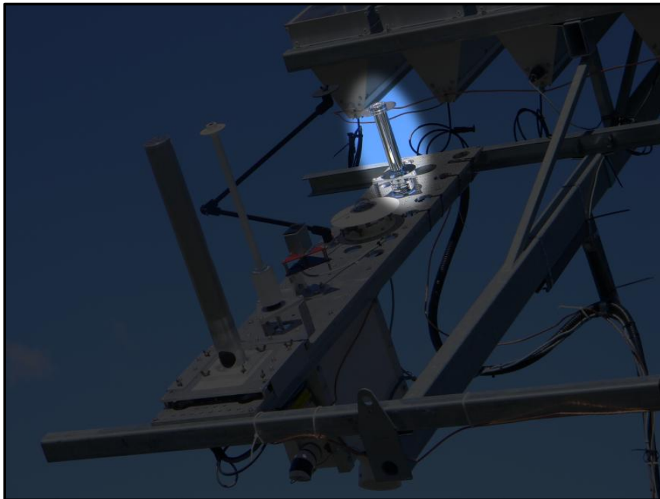
Figure 3-2: The highlighted instrument is the pyrhelimeter mounted on the SUNRISE demonstrator. The pyrhelimeter is used to measure the total incident power of the direct portion of the insolation.
