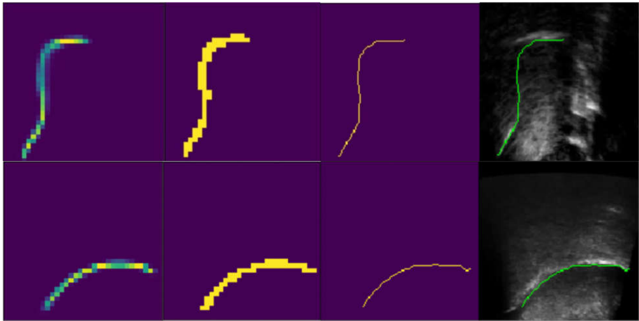
Figure 6-5 The postprocessing steps: from raw prediction array (left) to binarized mask (second), the extracted skeleton (third) and the final superimposed image (last)
