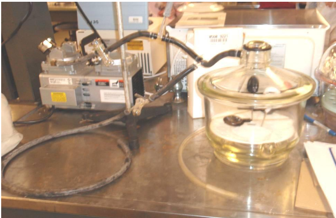
Figure 3.1 (b) the vacuum desiccator systems for the adsorption vacuum evaporative cooling (AVEC) tests
