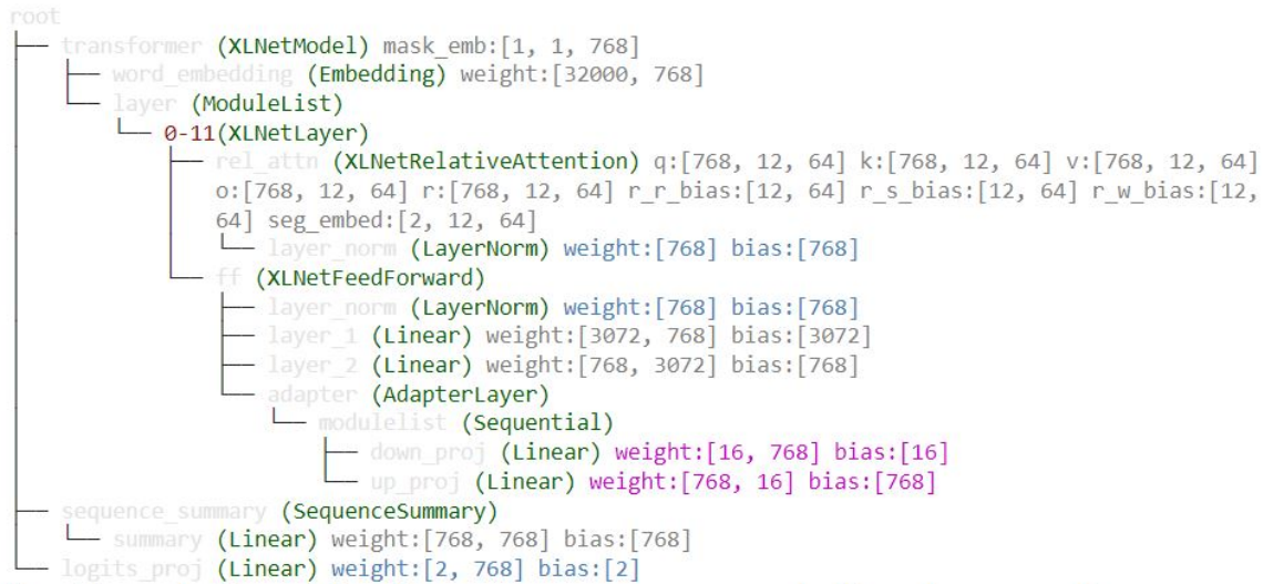
Figure 4.6: The Alternative Architecture of XLNet with Adapter Tuning
