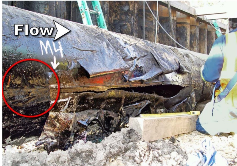
Figure 1.4 The ruptured pipe segment of Line 6 in the oil spilled accident at Marshall, Michigan on July 25, 2010.
