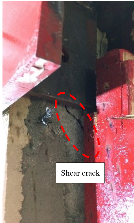
Figure 5-15. R-C-N: Premature Shear cracks at 3 rd shot (Jung, 2020)
