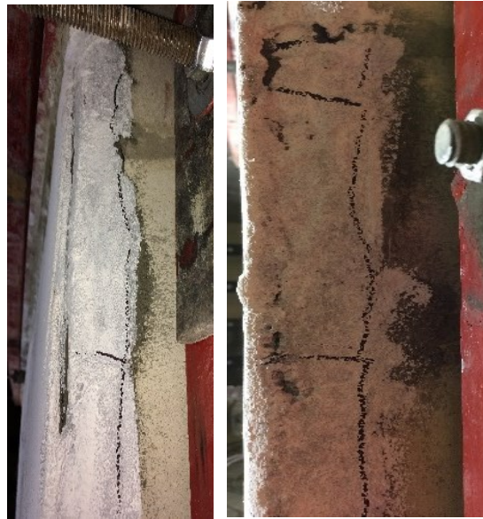
Figure 5-12. Visible Debonding on R-S-L, 5 th shot (side), (Jung, 2020)
