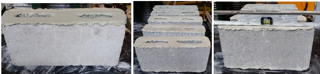
Figure 3-14. Leveling and capping of the specimens with high strength mortar
