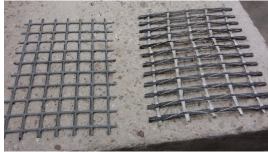
Figure 2-4. FRCM carbon grid: Bidirectional (left) and unidirectional (right) (taken from manufacturer’s data sheet)
