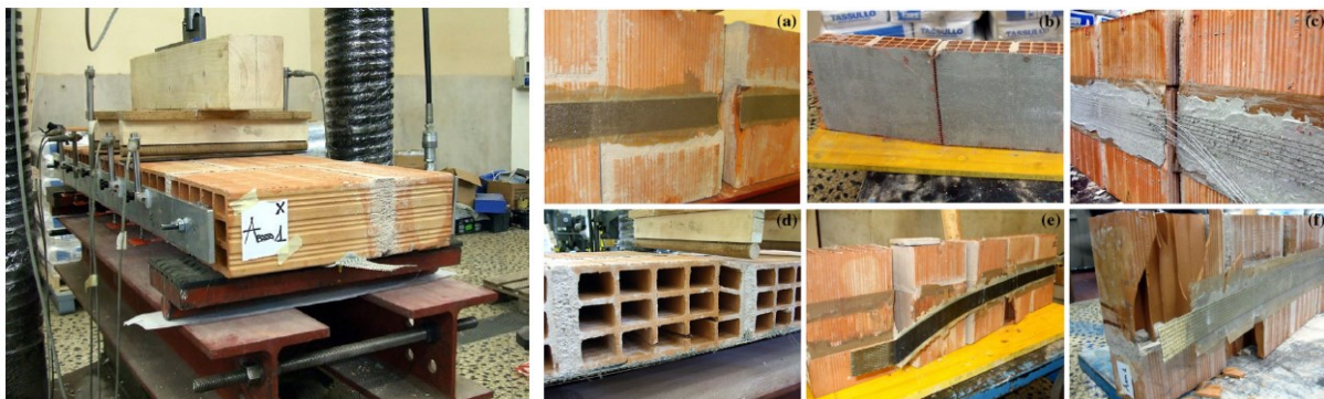
Figure 2-9. Test setup and failure modes, Tensile rupture of a) Flax FRP and b) Plaster net; c) splitting of fibres; d) shear failure in Basalt TRM; debonding in e) Basalt FRP and f) HD SRP (Valluzzi et al., 2014)
