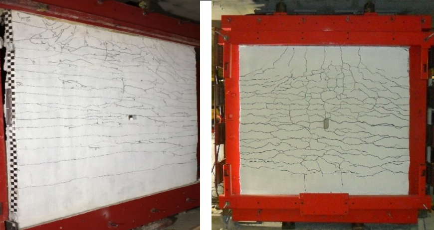
Figure 5-17. Axial Effect on CMU Walls, Performance Comparison:RCL-YC-3 vs R-C-N (R-C-N data from Jung, 2020)
