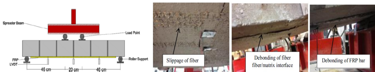
Figure 2-11. Test setup and results (Al-Jaberi et al., 2018)
