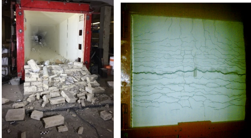
Figure 5-14. Load-Bearing Walls (CMU vs Stone), Retrofit Comparison: RCL-YC-3 vs R-S-L (R-S-L data from Jung, 2020)
