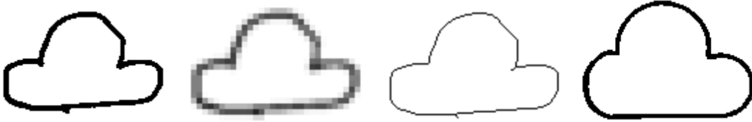
Figure 3.15 - Input image, a pixelated input image, a skeletonized input image, and GANdex corrective vector of the input image
