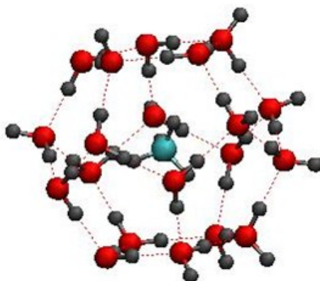
Figure 3.2: Single clathrate hydrate cage encapsulating a methane molecule. Hydrogen bonds between water molecules are represented by dotted lines.
