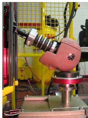
Figure 3. Unhelmeted Hybrid III head and neckform attached to monorail drop rig and impacting a MEP anvil.
