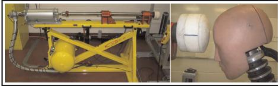
Figure 1. Linear impactor prior to pneumatic release (left); unhelmeted Hybrid III head- and neckform immediately prior to striker contact.
