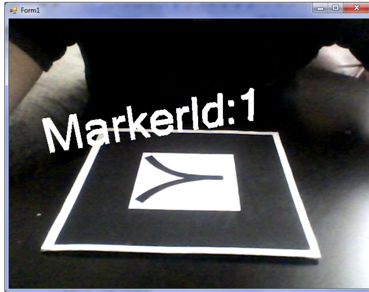
Figure 8: Virtual text overlaid on a marker detected in the environment
