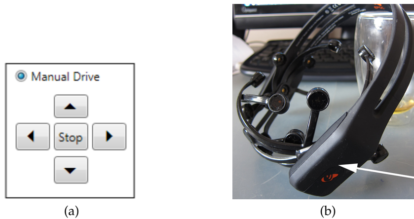
Figure 24: a) The UI buttons used with the BCI as mouse control method b) location of the gyroscope on the acquisition device
