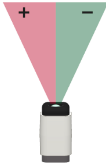
Figure 4. 9 The field of view of PIR NIS1070
