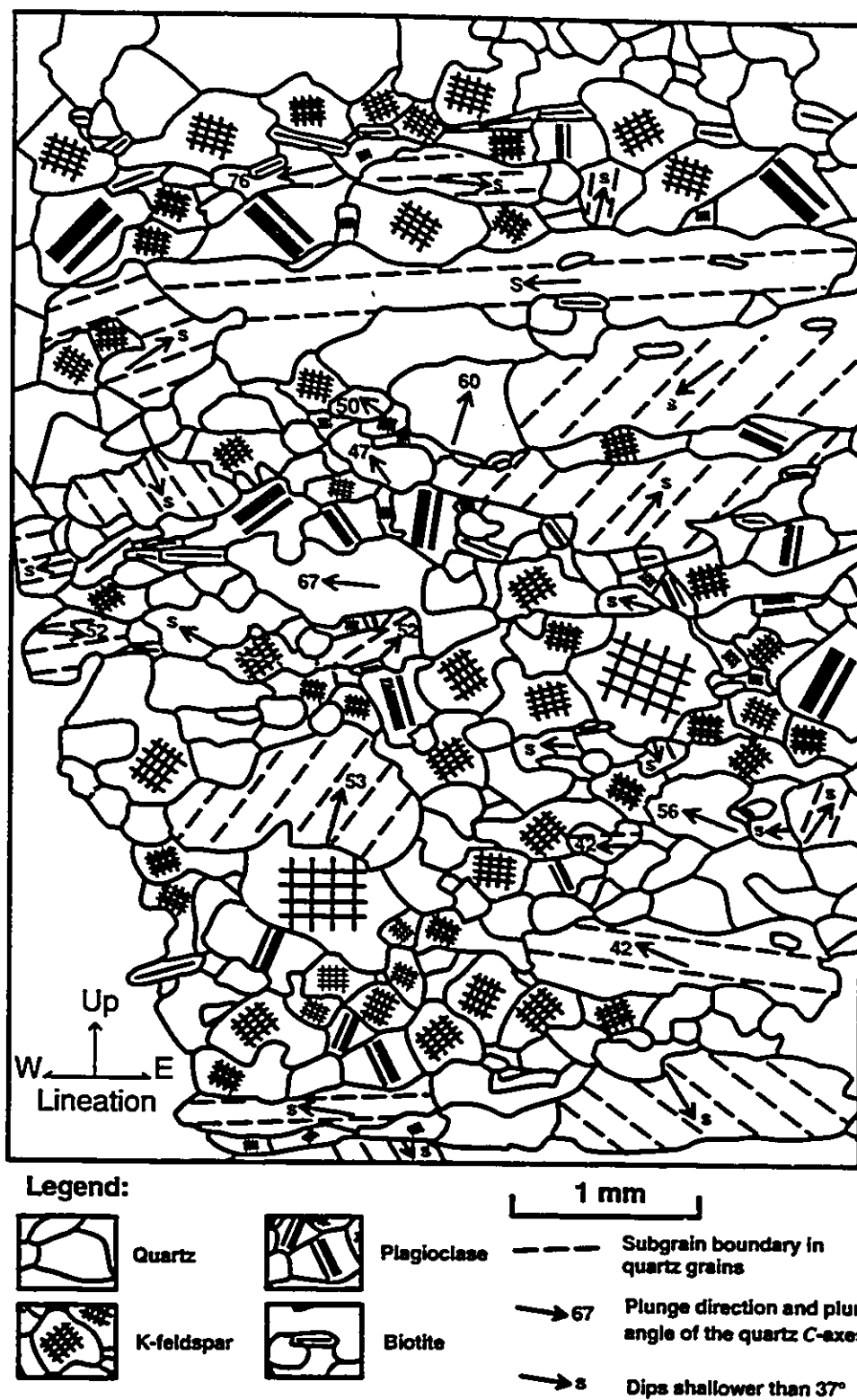
Fig. 3.5. Microfabric map of part of a thin section from the Lac Opasatica gneiss. Note the relationship between the subgrain boundaries and orientation of the quartz c-axes.
