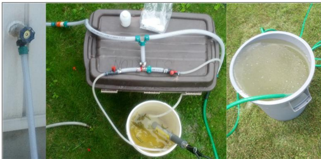
Figure 3-2. Sampling apparatus used to collect groundwater samples from privately owned wells.
