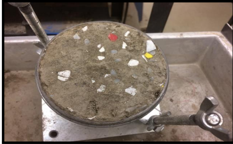
Figure 7.14 . Soil sample with flakey type of plastic for moisture testing
