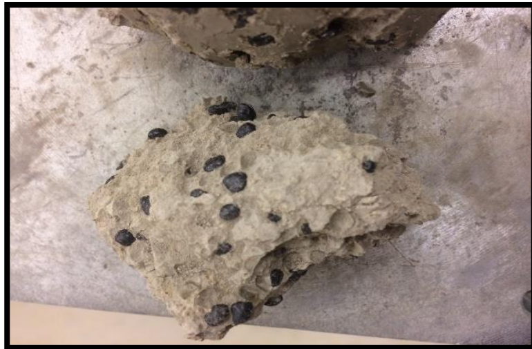
Figure 7.15. Soil sample with pellets type of plastic for moisture testing
