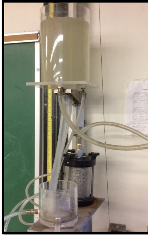
Figure 7.12. Device used for Permeability test
