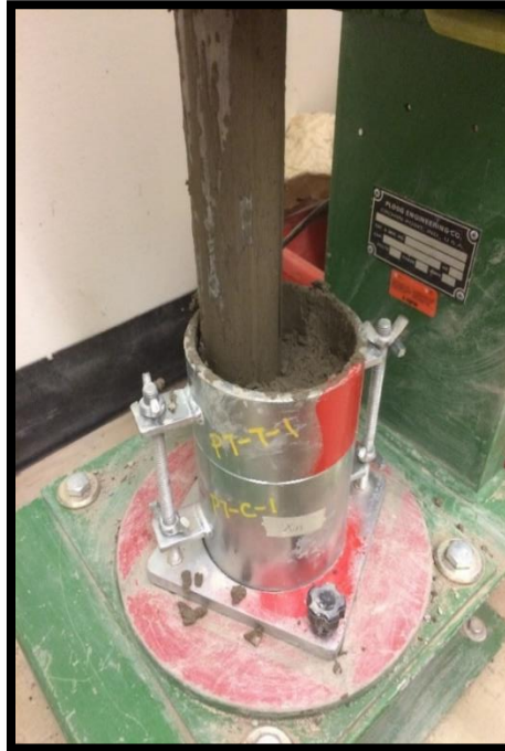
Figure 7.8. Automated proctor compactor
