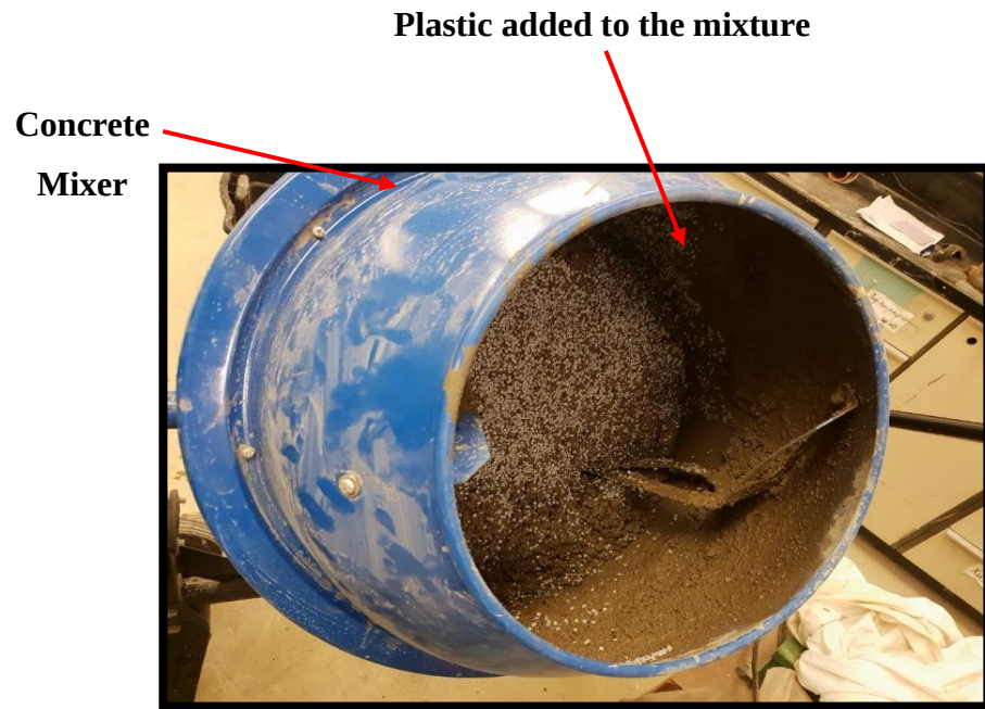
Figure 7.16. Concrete mixer and mixing process of concrete with plastic
