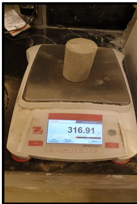
Figure 7.21 Shear samples being weighed
