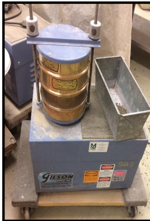
Figure 7.5. Sieve shaker used for grading analysis
