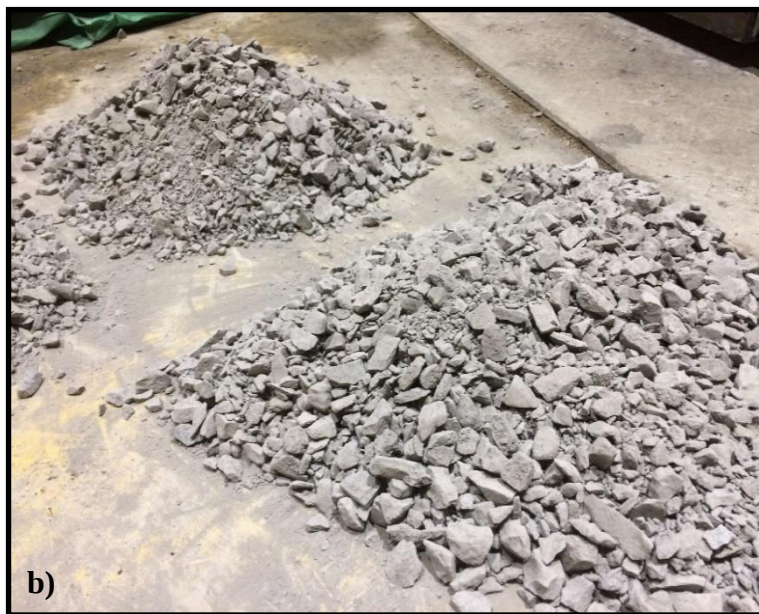
Figure 4.19. (a) Production of the granular material at the quarry, and (b) the as-received granular material used for the investigation
