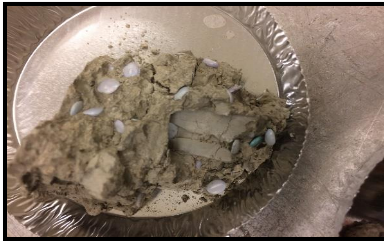
Figure 7.13. Soil sample with pellets type of plastic for moisture testing
