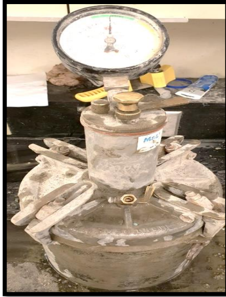
Figure 7.20. Aerometer for measuring air content of fresh mixture
