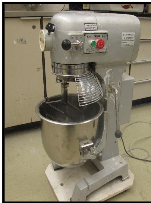
Figure 7.7. mixer for preparing Sub-base and base batches for later testing
