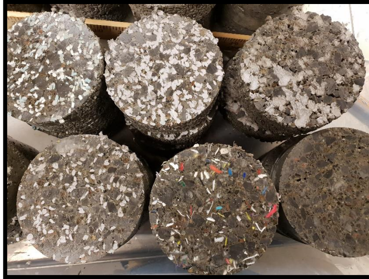
Figure 7.26 Cylinder samples for capillary testing
