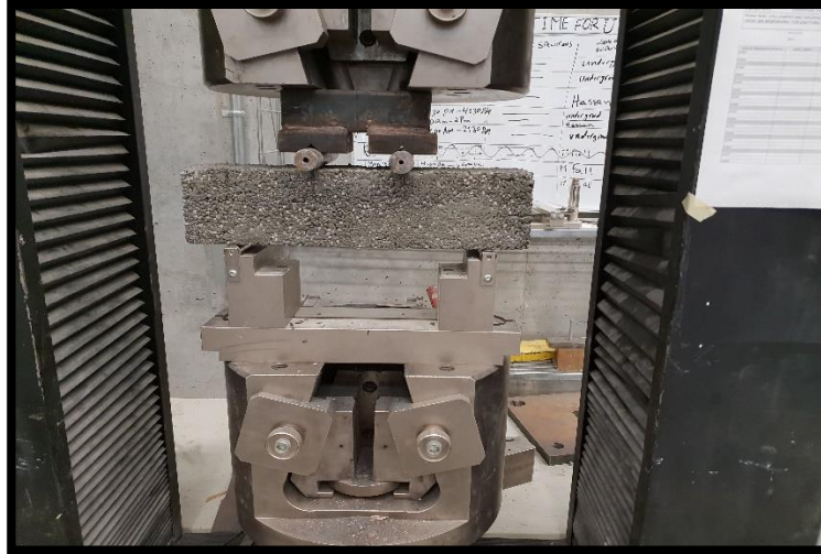
Figure 7.24 Concrete beam ready for flexural testing
