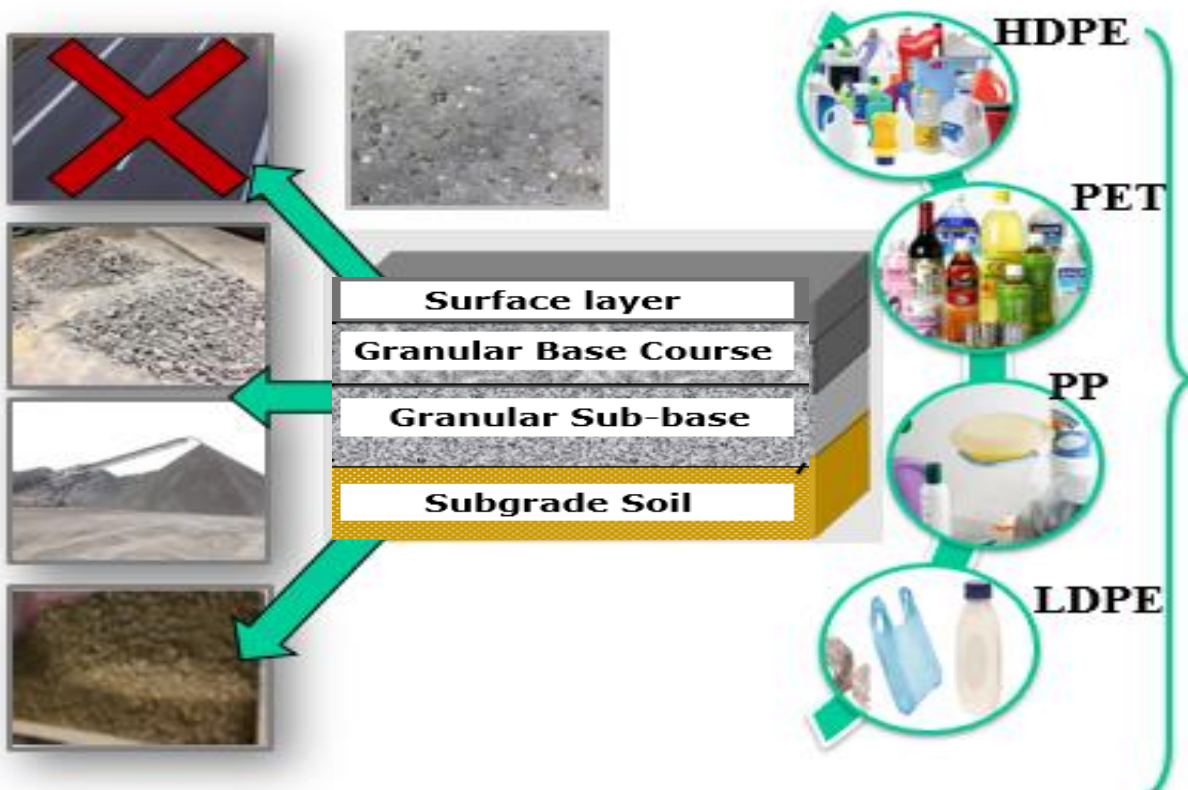
Figure 4.1 Structure of the studied pavement layers and incorporated materials of the research study
