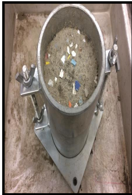
Figure 7.9. Sample inside proctor mold after compaction
