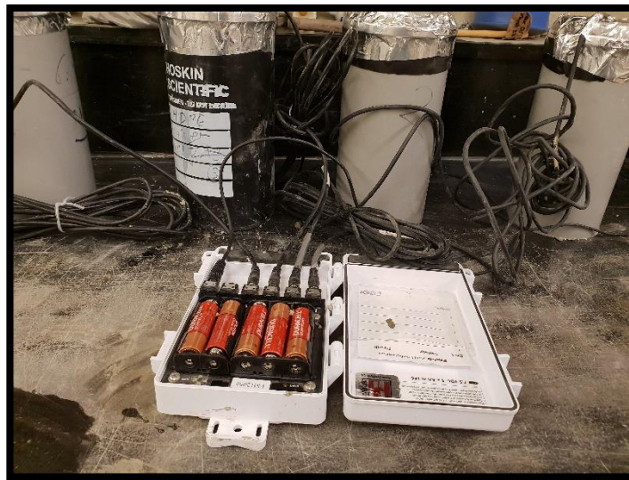
Figure 7.27 Samples casted in cylinders and connected to data acquisition for conductivity testing
