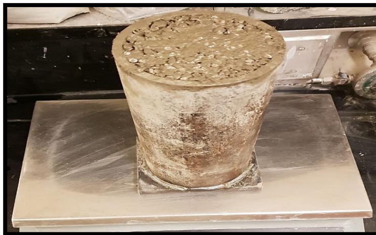
Figure 7.19. measuring density of fresh concrete
