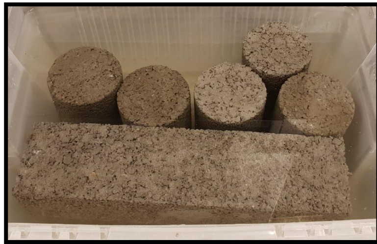
Figure 7.17. Illustration of samples curing in water prior to testing
