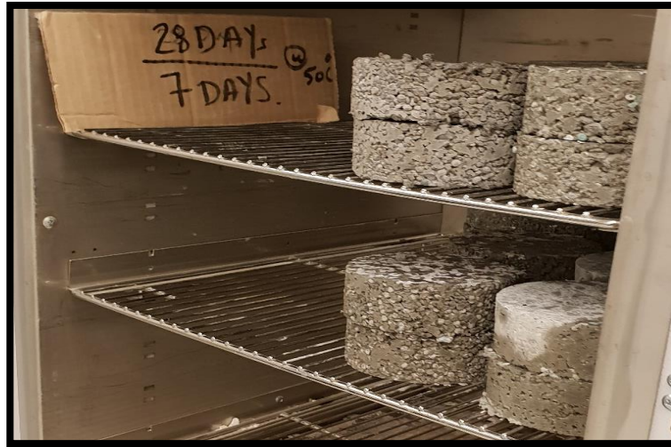
Figure 7.22. Samples in oven being prepared for density testing
