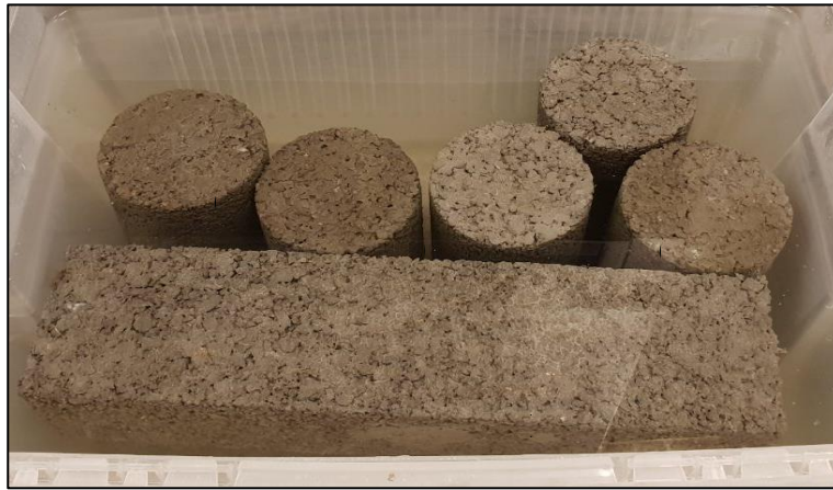
Figure 4.43. Illustration of samples curing in water prior to testing
