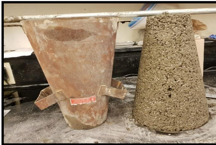
Figure 7.23. Zero slump concrete mixtures
