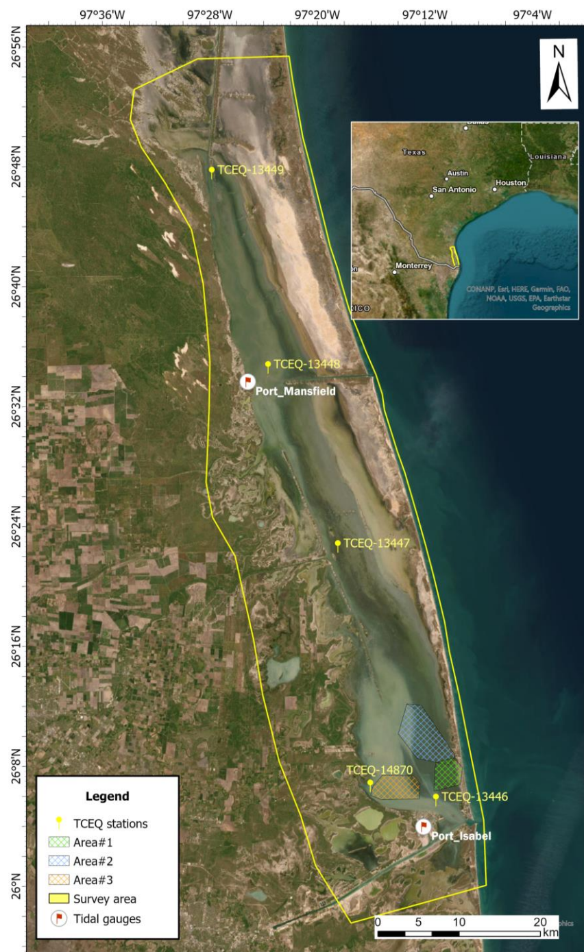
Figure 4-2. Lower Laguna Madre in southern Texas and in-situ locations (TCEQ reference stations, NOAA tide gauges, and BEG observation areas). The yellow polygon indicates the extent of the airborne survey area (1600 km 2 ).
