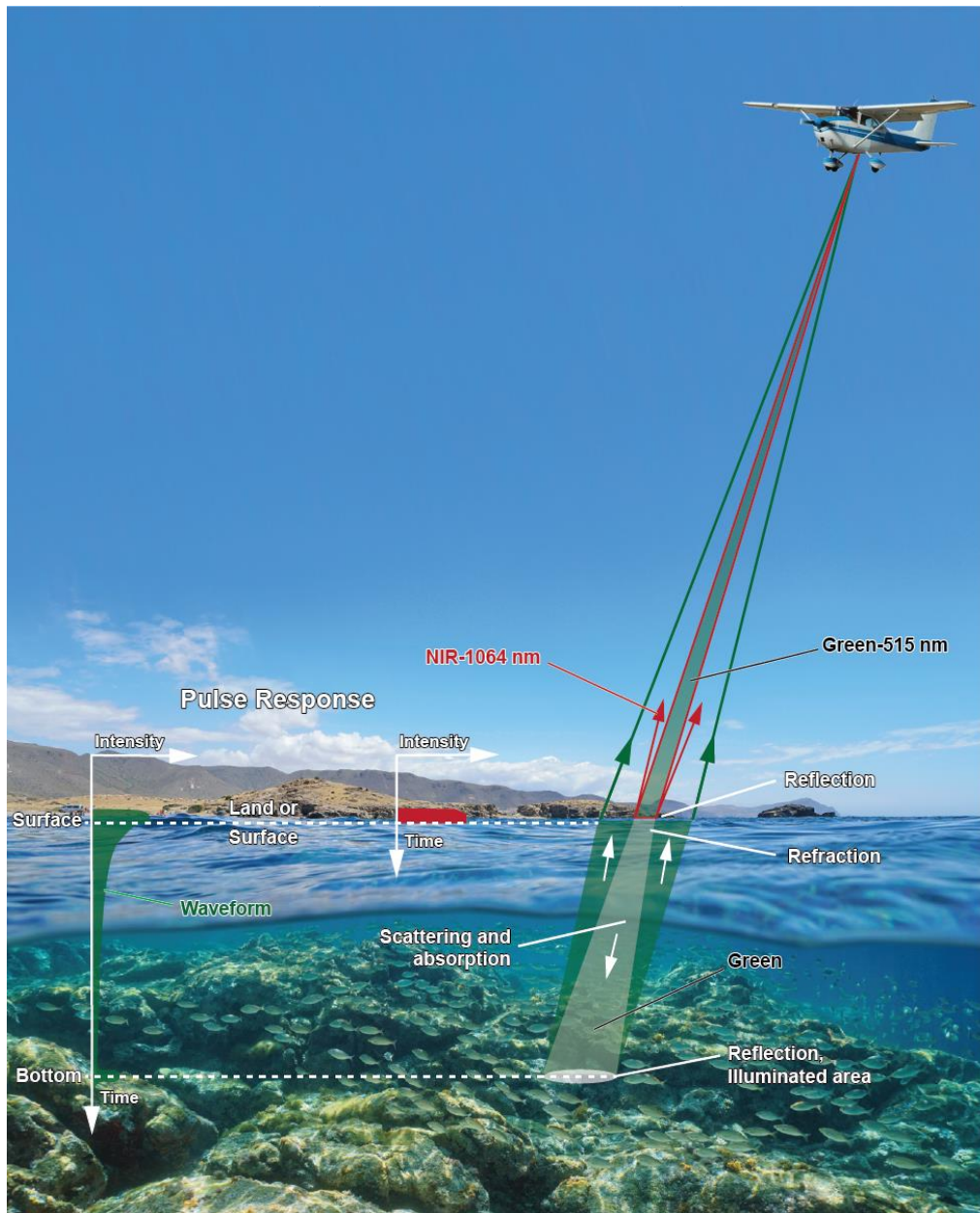
Figure 3-1. Scattering and refraction occur when light beams traverse through the air–water interface. Near infrared (NIR) beams are absorbed either at the surface or in the immediate water column, whereas some reflect to the receiver and indicate the water surface. Distances (range) from the surface and bottom can be computed by measuring the flight duration of the pulses and adjusting the varying speed of light in air and water.
