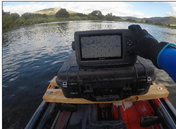
Figure 3-6. Surveying stream depth using a dual-beam Garmin echosounder.
