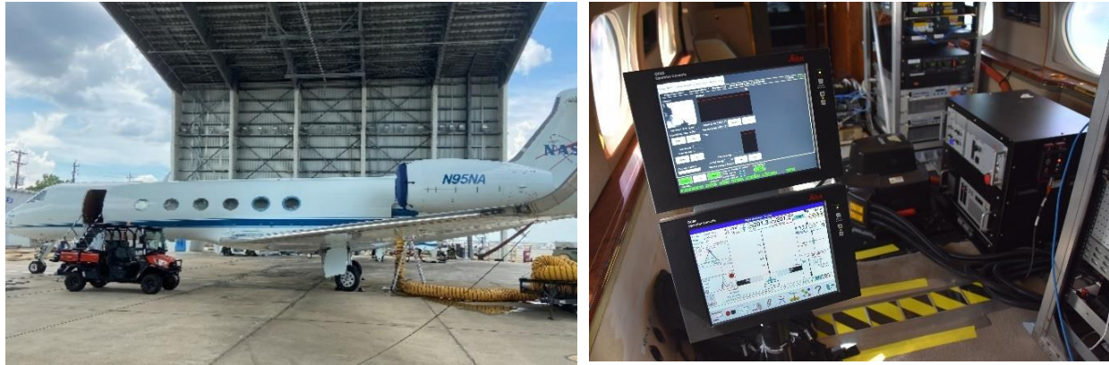
Figures 5-4 (a, b): CHIR and LVIS were installed onto a Gulfstream V (N95NA) aircraft at Ellington Field in Houston, Texas. This aircraft had a pressurized cabin and two glass viewports, where both instruments were mounted.
